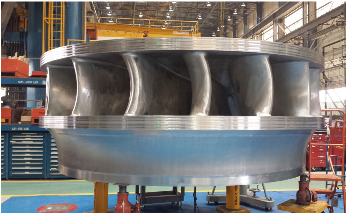
Photo showing turbine runner being installed at the Trinity Powerplant, which will increase the power-generation efficiency.
