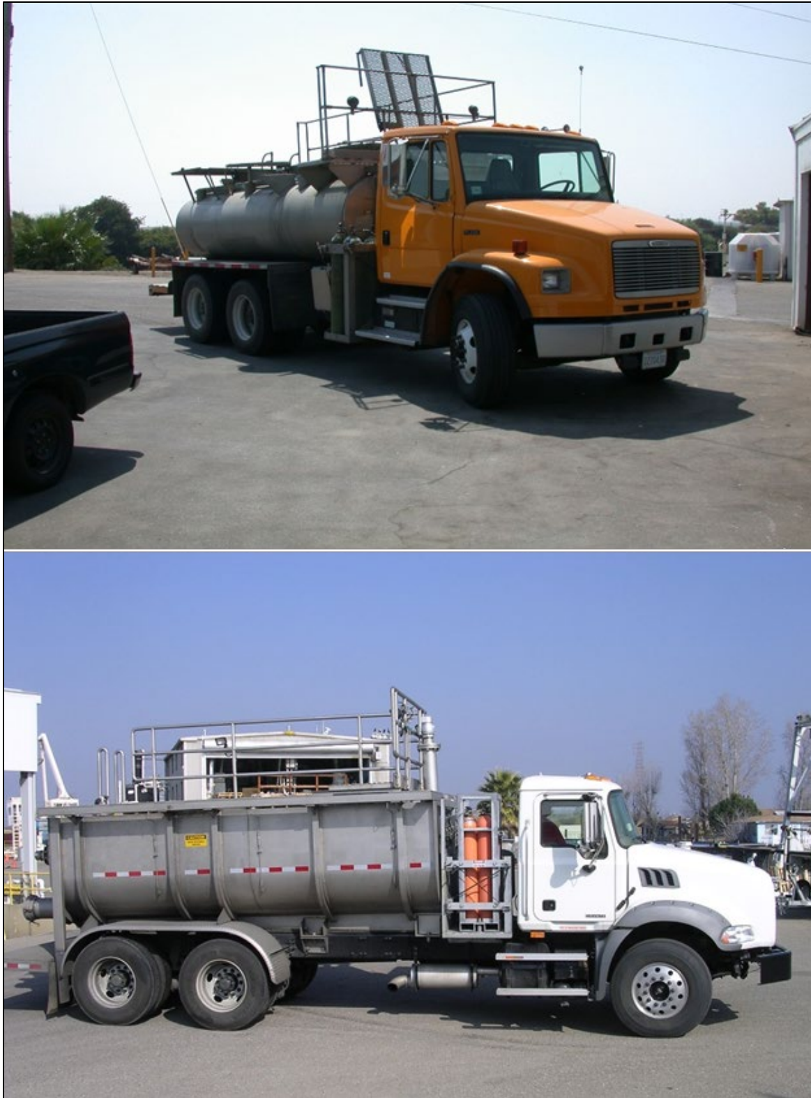
Figure 2.—Third-generation fish-haul truck (7,570.8-L; equipped with oxygen [O 2 ] system only) historically used (1990–2008) to transport fish from the Tracy Fish Collection Facility (TFCF) to fish release sites (top) and fourth-generation fish-haul truck (9,914.0-L; equipped with compressed air and O 2 systems) currently used (2008–present) to transport fish from the TFCF to fish release sites (bottom).
