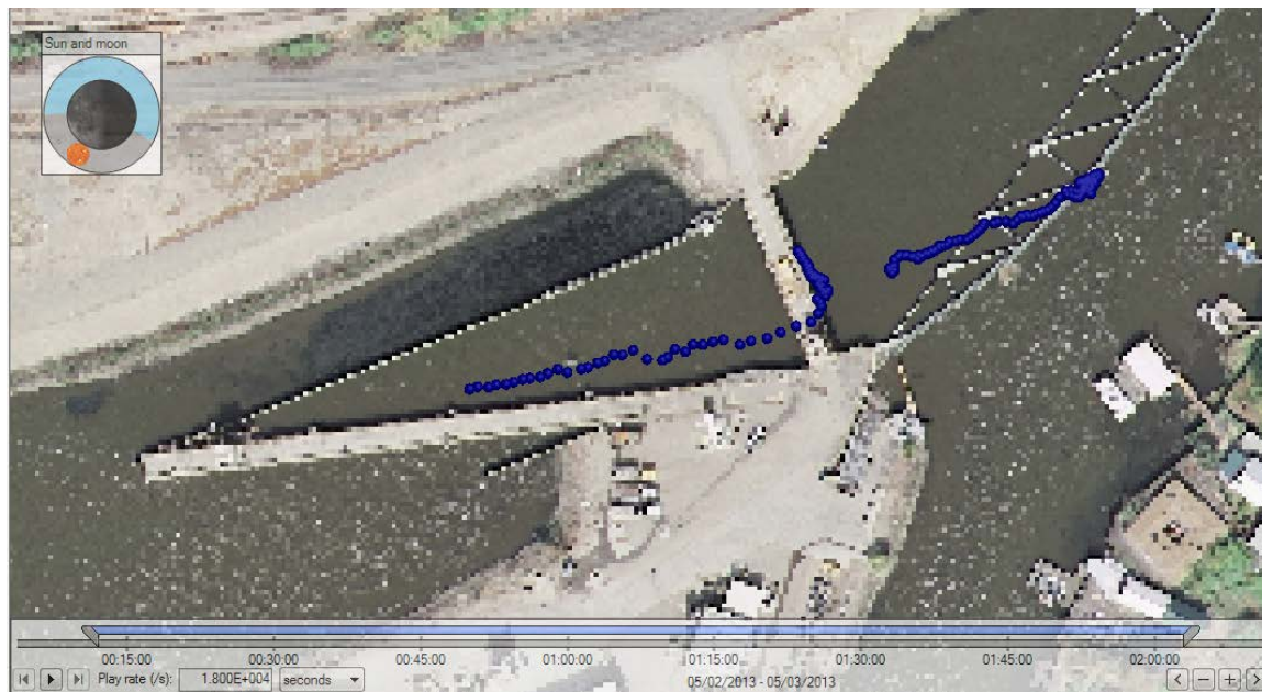
Figure C-26. Track of Chinook salmon 3379 (released at high flow, total time in system was about 10 min: 2 min in the upstream channel, 2 min along the trash rack, 1 min in the primary channel, and 5 min in the bypass pipes/secondary channel).
