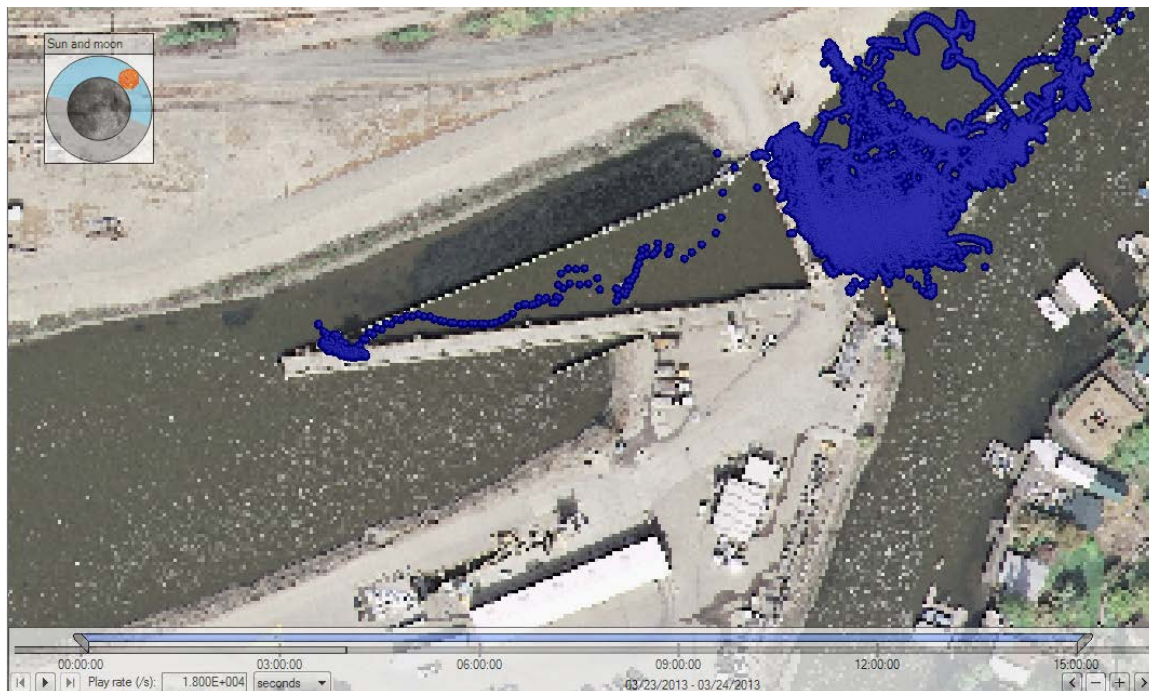
Figure C-2. Track of Chinook salmon 2315 (released at low flow, total time in system was 13.7 h: 10 min in the upstream channel, over 13 h along the upstream side of the trash rack, about 10 min in the primary channel, and 44 min in the bypass pipes/ secondary channel).
