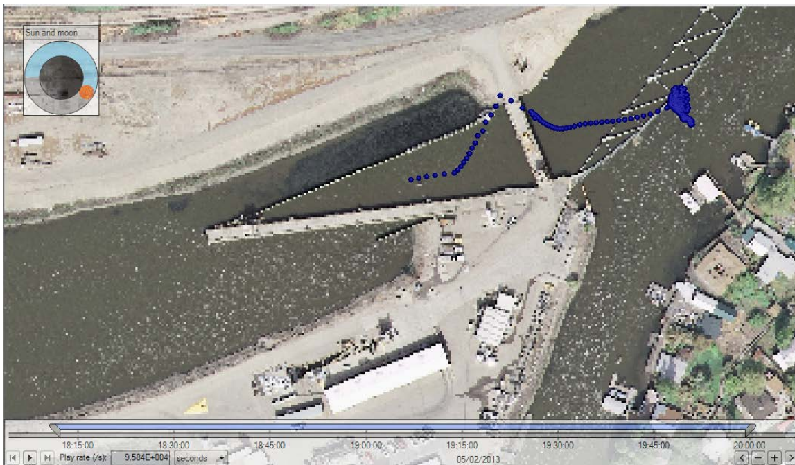
Figure C-21. Track of Chinook salmon 3071 (released at high flow, total time in system was about 7 min, mostly in the bypass pipes and secondary channel).
