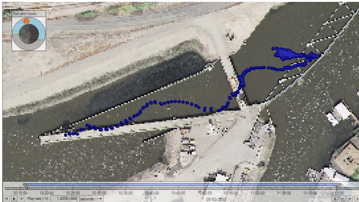
Figure C-22. Track of Chinook salmon 3211 (released at high flow, total time in system was about 40 min: 11 min in the upstream channel, 1 min along the trash rack, 2 min through the primary channel, and 26 min in the bypass pipes/secondary channel).
