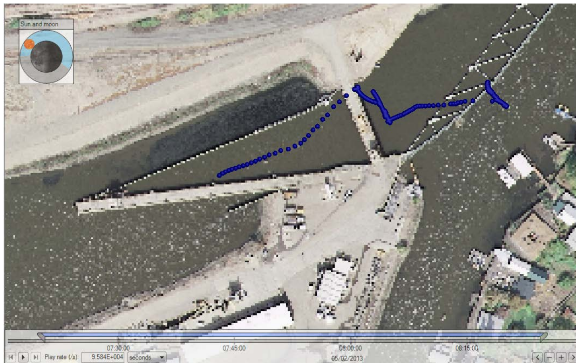
Figure C-24. Track of Chinook salmon 3295 (released at high flow, total time in system was about 20 min: 2 min in the upstream channel, 1 min along the trash rack, 13 min in the primary channel and 4 min in the bypass pipes/secondary channel).
