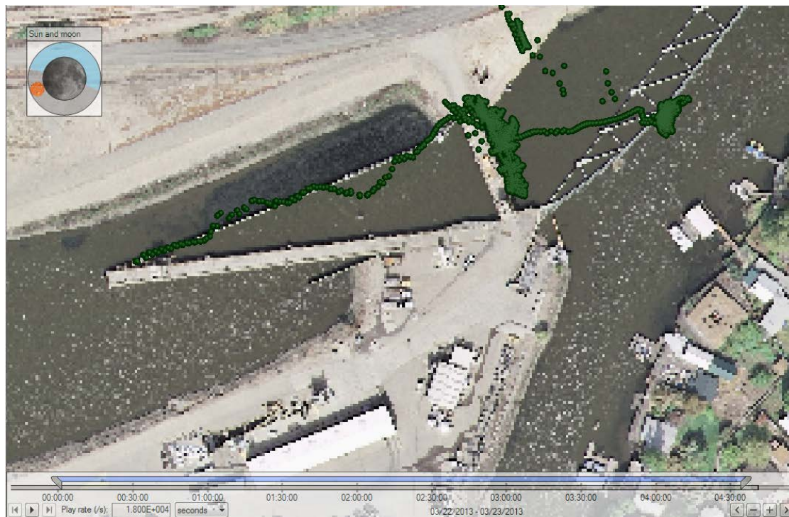
Figure C-28. Track of steelhead 3127 (released at intermediate flow, total time in system was about 2.5 h: mostly along the upstream side of the trash rack).
