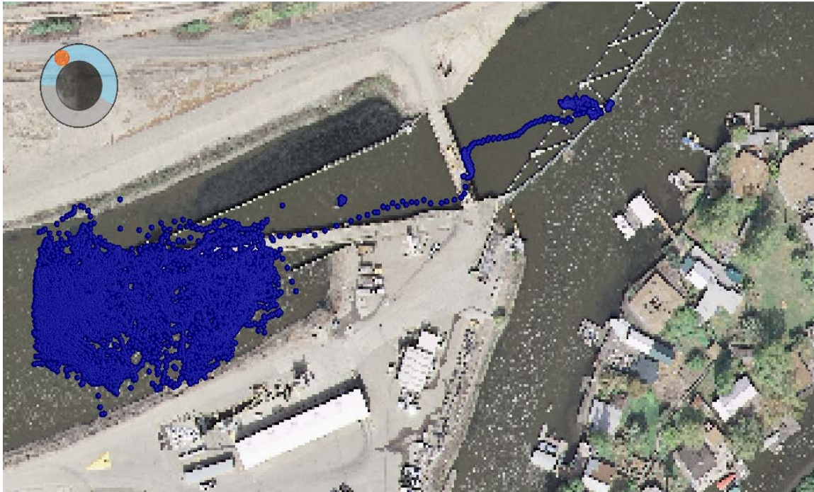
Figure 7. Example of primary louver loss of a Chinook salmon (fish was released during high flow experiment and passed through primary louver about 16 min later not during a cleaning event).
