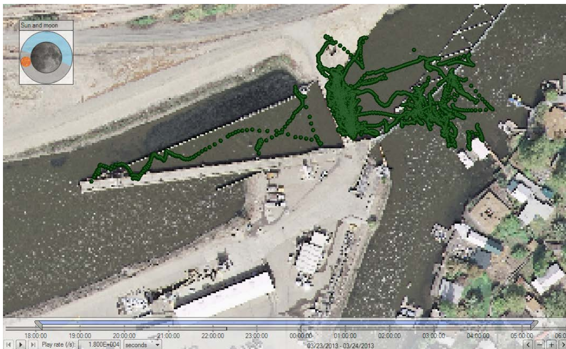
Figure C-27. Track of steelhead 2203 (released at low flow, total time in system was about 9 h: 17 min in the upstream channel, over 8 h in front of the trash rack, 11 min in the primary channel and 3 min in the bypass pipes/secondary channel).
