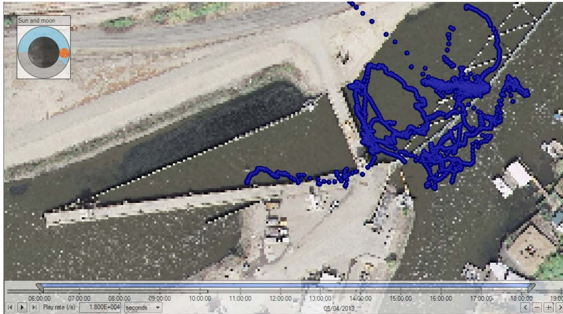
Figure C-1. Track of Chinook salmon 2091 (released at low flow, total time in system was over 10 h, mostly in upstream channel and along the upstream side of the trash rack).
