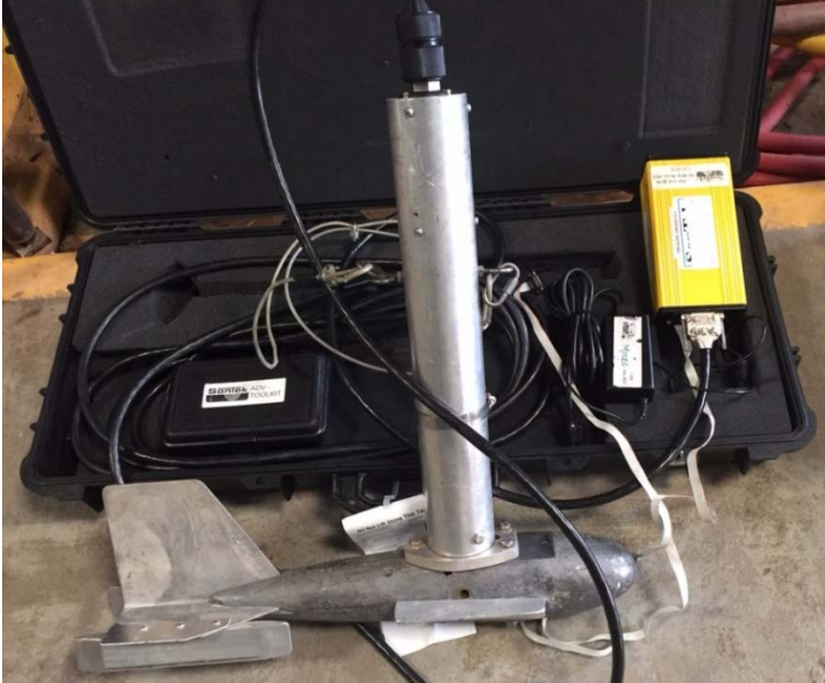
Figure 5. SonTek/YSI Micro ADV deployment setup used for the Hydrolox screen evaluation. The ADV probe is mounted inside a 2-in diameter aluminum tube. The sounding weight maintains the ADV position into the flow and offset 3 in from the screen face.
