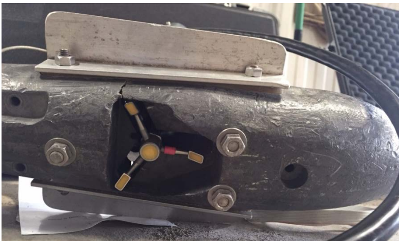
Figure 6 Close-up view of the SonTek Micro ADV probe's orientation inside the sounding weight. The arm with the red tape indicates the x-axis for this probe.
