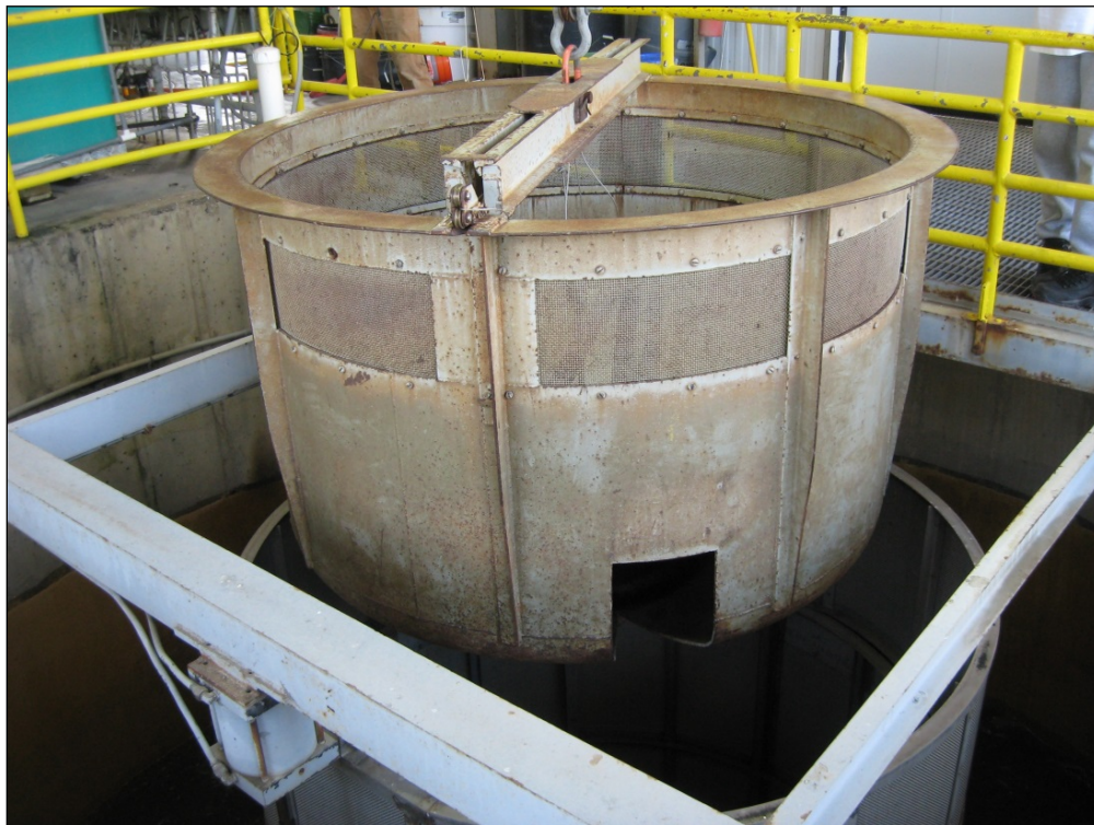
Figure 2.—Fish transfer bucket (1,544-L, 408-gal), Tracy Fish Collection Facility, Byron, California.
