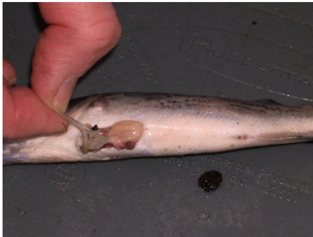
Figure 3.—External injuries observed in traveling screen experiments.
