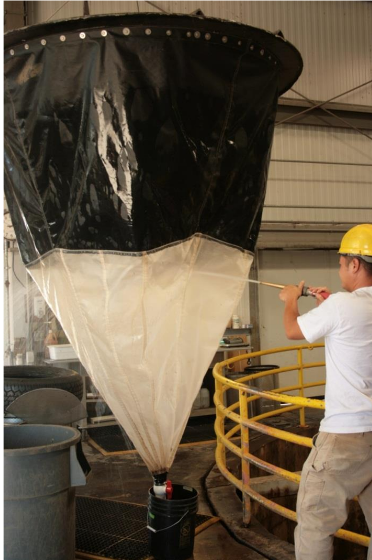
Figure 6.—Contents of 500- \mu\text{m} net being rinsed into 18.9-L bucket to recover fish during evaluation of Tracy Fish Collection Facility (Bureau of Reclamation, Byron, California) holding tank screen retention efficiency for 20–30 mm fork length juvenile delta smelt during 30-minute collection periods.
