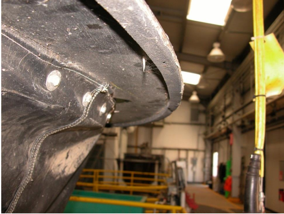
Figure 4.—Rubber foam weather stripping (1.9-cm wide by 1.1-cm thick) attached to outside, bottom lip of steel frame used, along with a 500- \mu m net, to test retention efficiency of Tracy Fish Collection Facility (Bureau of Reclamation, Byron, California) holding tank screens for 20–30 mm fork length juvenile delta smelt during 30-minute collection periods.
