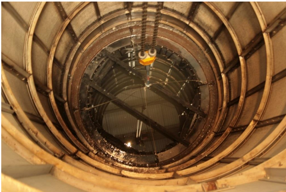
Figure 5.—The 500- \mu m net and frame seated in holding tank drainage pit at the Tracy Fish Collection Facility (Bureau of Reclamation, Byron, California).
