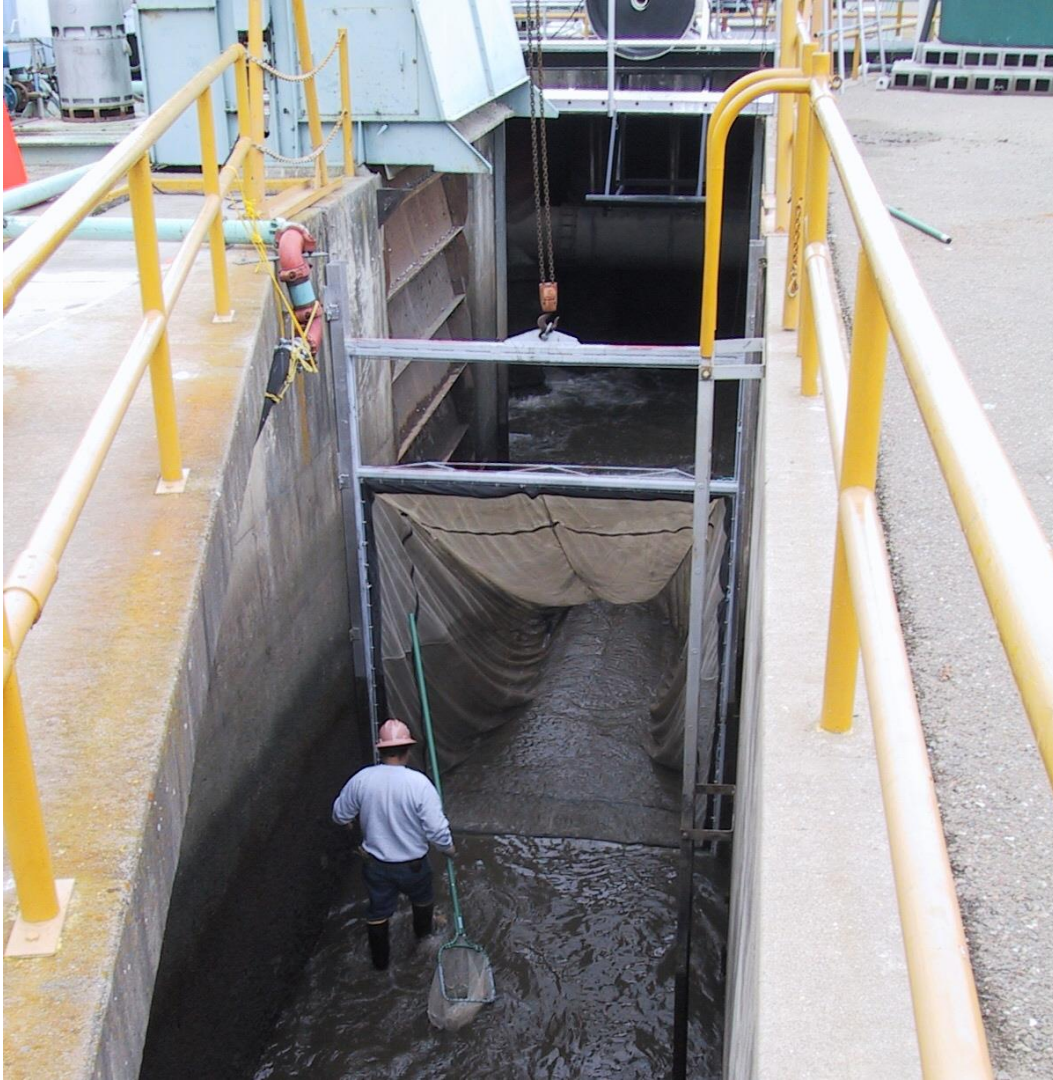
Figure 4.—Sieve net used downstream of the secondary louver arrays at the Tracy Fish Collection Facility to capture adult and juvenile delta smelt ( Hypomesus transpacificus ) that passed through the louvers.
