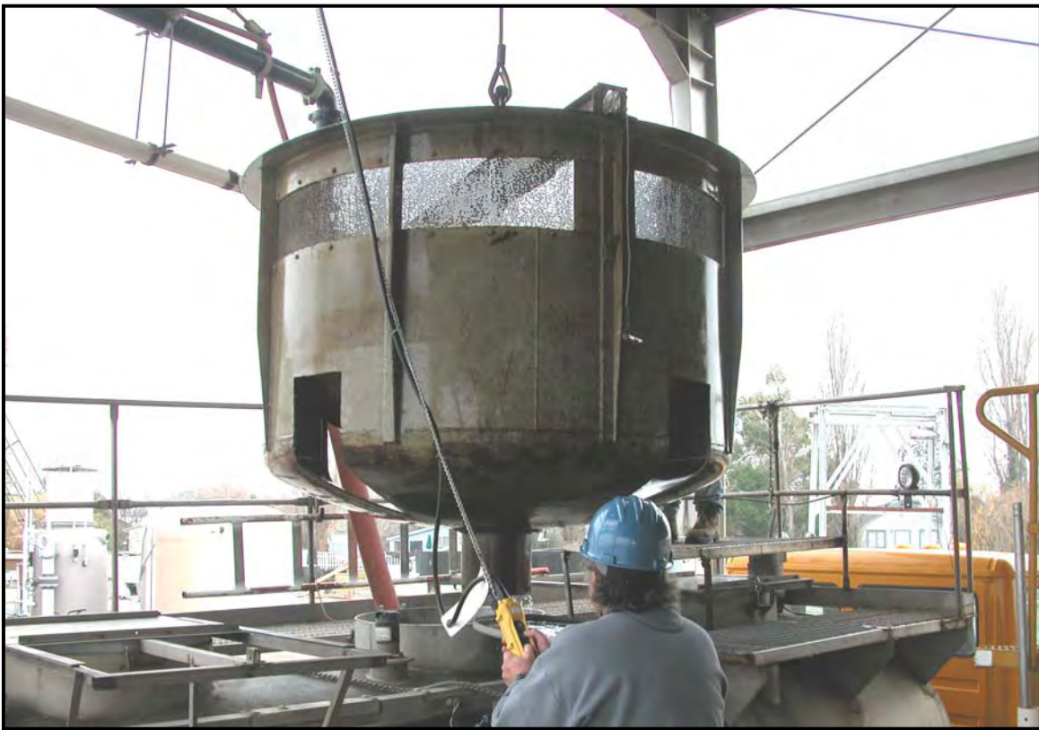
FIGURE 4.—The Tracy Fish Collection Facility fish haul-out bucket.
