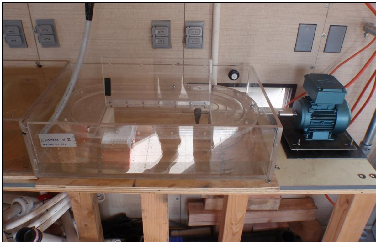
Figure 5.—Fish swimming flume (24" long × 10" wide × 5" deep) and external variable speed 120V/60Hz motor (SEW-Eurodrive, Hayward, CA.) used to measure the swimming performance of fish during experimentation. Both swimming flumes are equipped with a fish swimming chamber, as well as a honeycomb filter, veins and cross-wings that aid in developing laminar flow.
