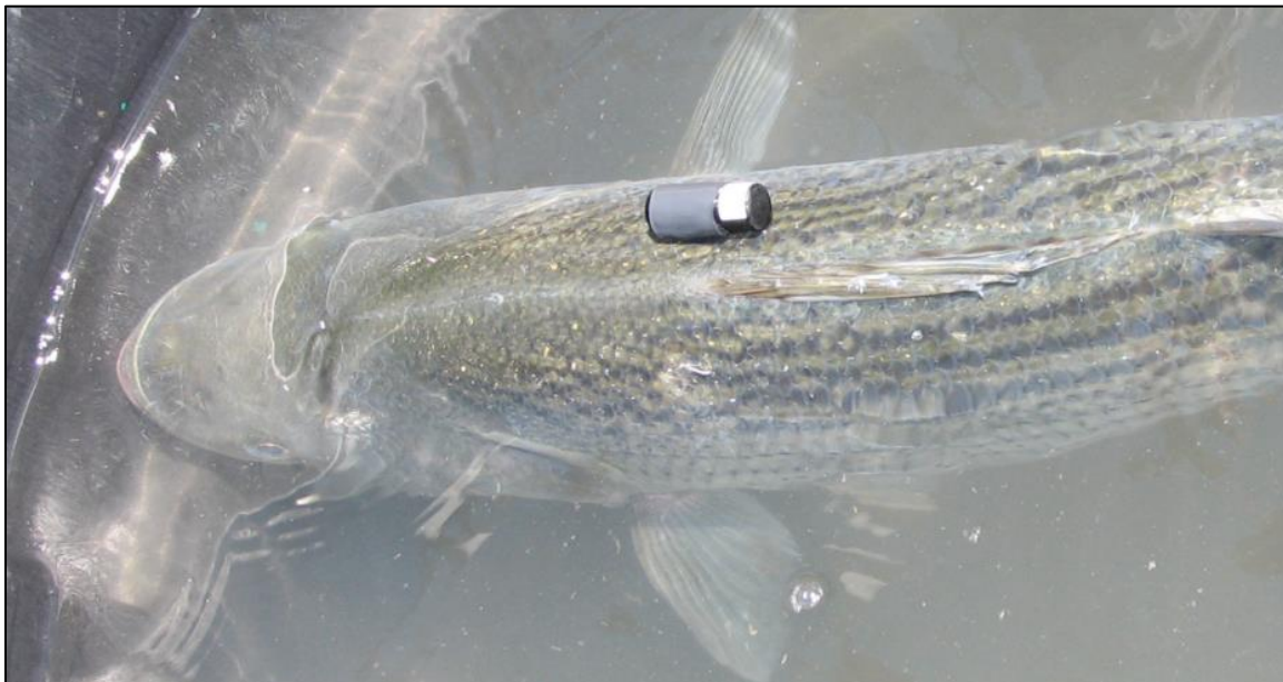
Figure 9.—A Striped Bass ( Morone saxatilis ) captured via hook and line sampling near the Curtis Landing Release Site in the Delta with an externally mounted VEMCO V13 acoustic transmitter. V13 acoustic transmitters were applied to 9 Striped Bass ( Morone saxatilis ) and one Sacramento Pikeminnow ( Ptychocheilus grandis ). Movement of predators with V13 tags was monitored using fixed and mobile hydrophones in the Sacramento San Joaquin River Delta in May 2017.
