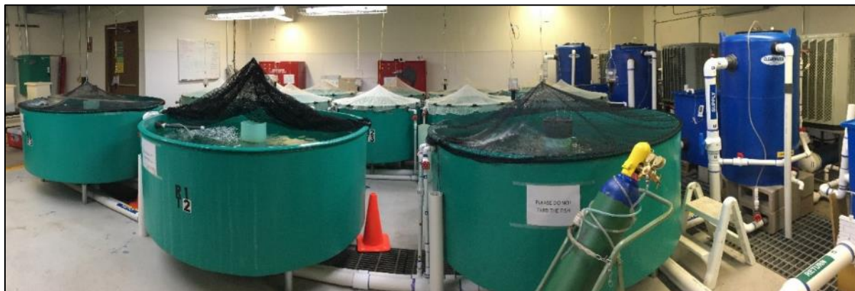
Figure 5.—Experimental tanks used for the March 2017 laboratory experiment at the Reclamation Technical Service Center Fisheries Laboratory in Denver, Colorado. Foreground holding tanks were used to hold bait fish, the background two rows were used for this experiment. Filters, heat pumps, and water pumps are seen on the right side of the figure.
