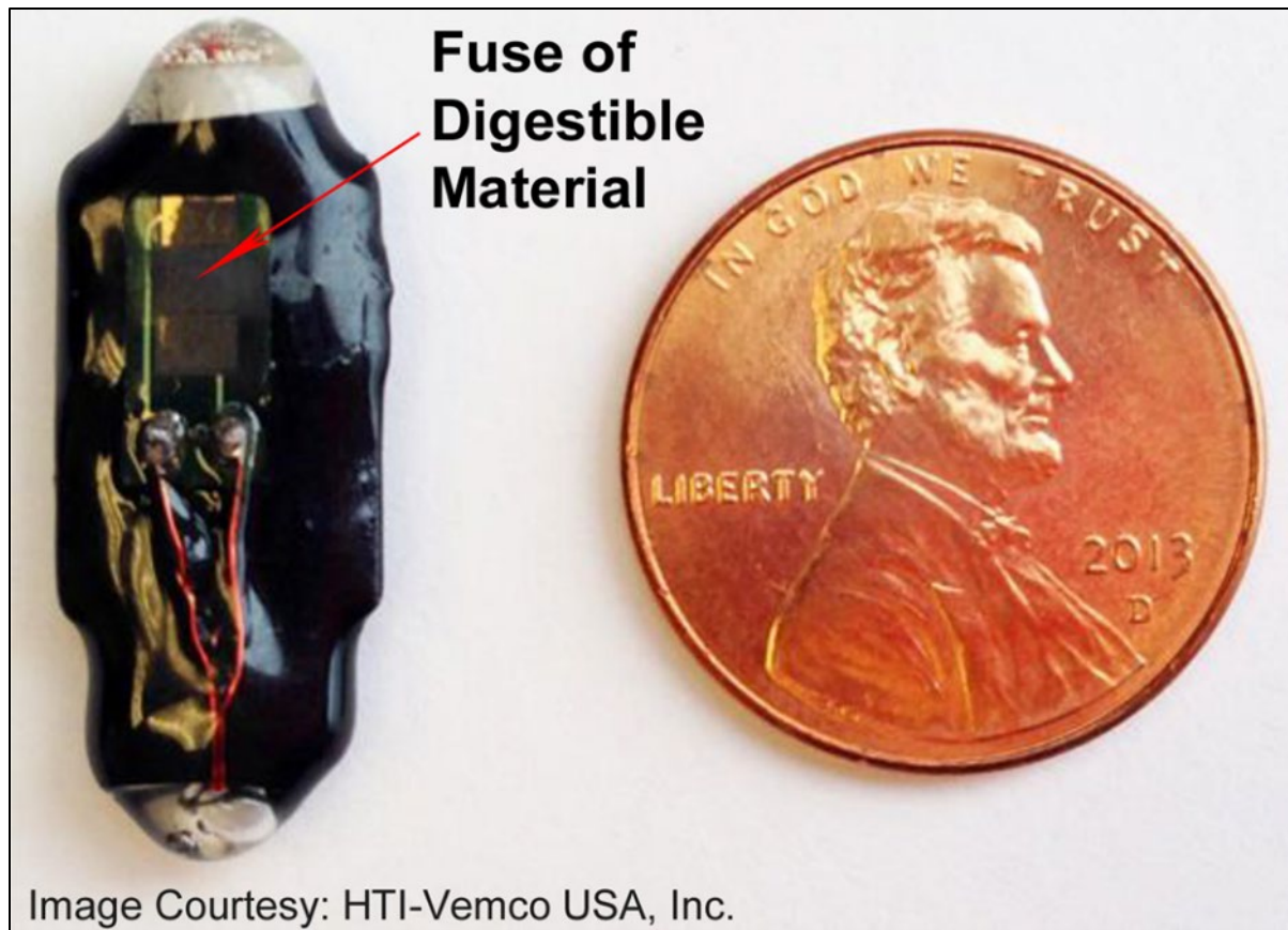
Figure 1.—Predation Detection Acoustic Tag (Model 900-PD; 307 kHz frequency; 1.0 g in air; 6.0-mm diameter x 25.0-mm long; HTI-Vemco USA, Inc., Seattle, Washington) with fuse of digestible material (polysaccharide and gelatin; image courtesy of HTI-Vemco USA, Inc.).
