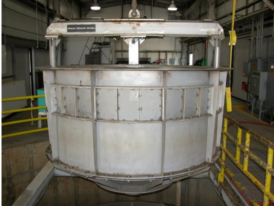
Figure 4.—Haul-out bucket (1544-L) used to transfer fish from holding tanks to the fish-haul truck during the haul-out process at the Tracy Fish Collection Facility.
