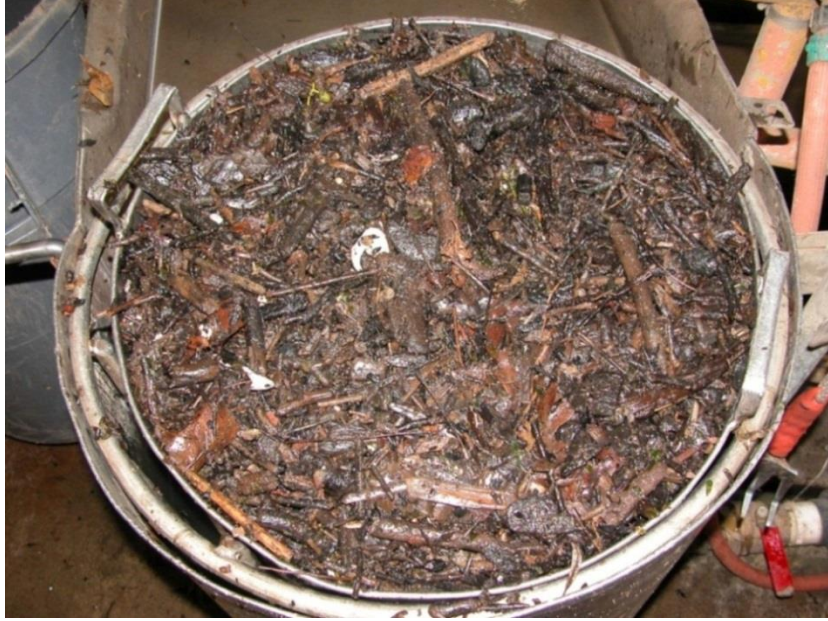
Figure 6.—Example of woody debris encountered during the salvage process at the Tracy Fish Collection Facility. Woody debris consisted mostly of sticks, twigs, roots, bark, seeds and peat during the Holding Tank Screen Lift evaluation.
