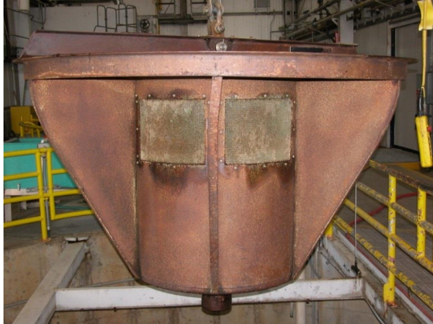
Figure 2.—Fish-count bucket (343-L) used to transfer fish from holding tanks to the fish-count station during salvage counts at the Tracy Fish Collection Facility.
