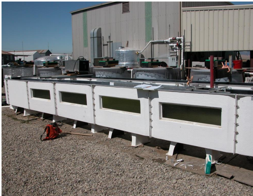
Figure 3.—Small oval flume (track width = 0.4 m, depth = 0.5 m, length = 8.2 m) used to examine fish swimming behavior with flowing water and elevated carbon dioxide concentrations at the Tracy Fish Collection Facility (top) and clear windows on the side of the flume for observing fish (bottom).
