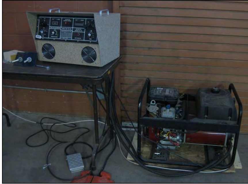
Figure 3.—Smith-Root GPP 9.0 electrofisher unit with gas powered generator.
