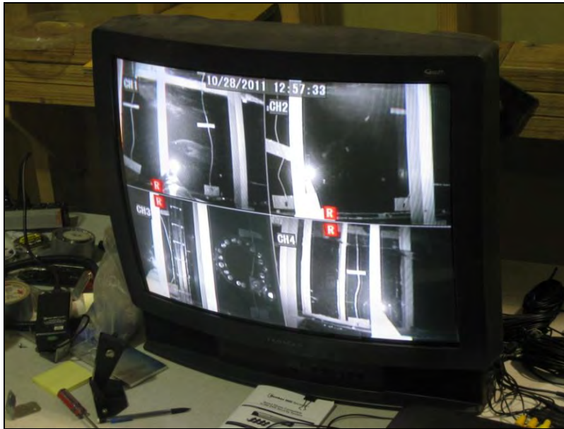
Figure 7.—Four remote infrared cameras were used to observe and document fish behavior.
