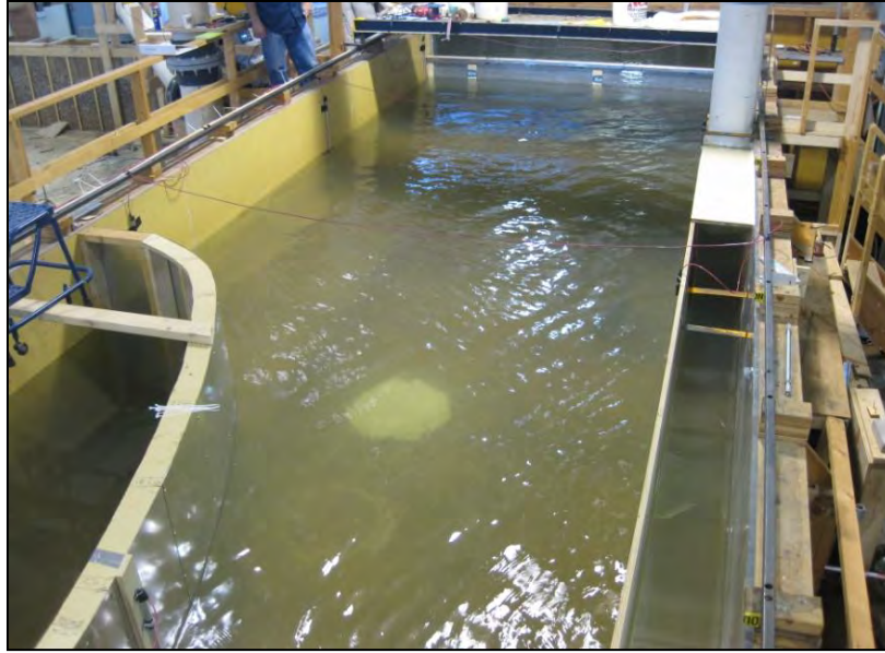
Figure 12.—Upstream view of flume showing the electrodes attached to the model sidewalls.
