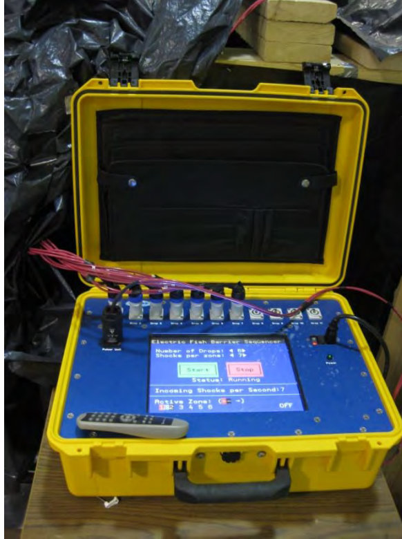
Figure 9.—A sequencer was developed to move the pulsed DC field to successive electrodes at a specified speed.
