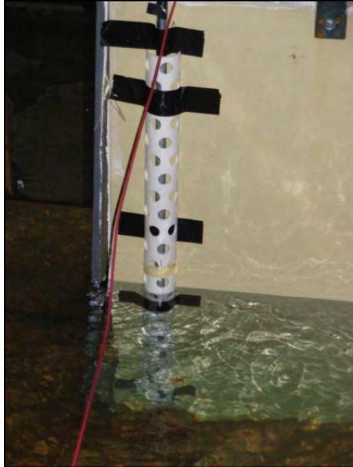
Figure 14.—PVC electrode cover with 2.5-cm-diameter (1-in-diameter) holes.
