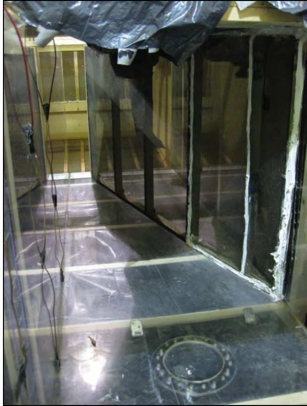
Figure 11.—After testing fish in a rectangular flume, the model was modified to include a screen angled at 15 degrees and a 15.2-cm-wide (6-in-wide) bypass opening.
