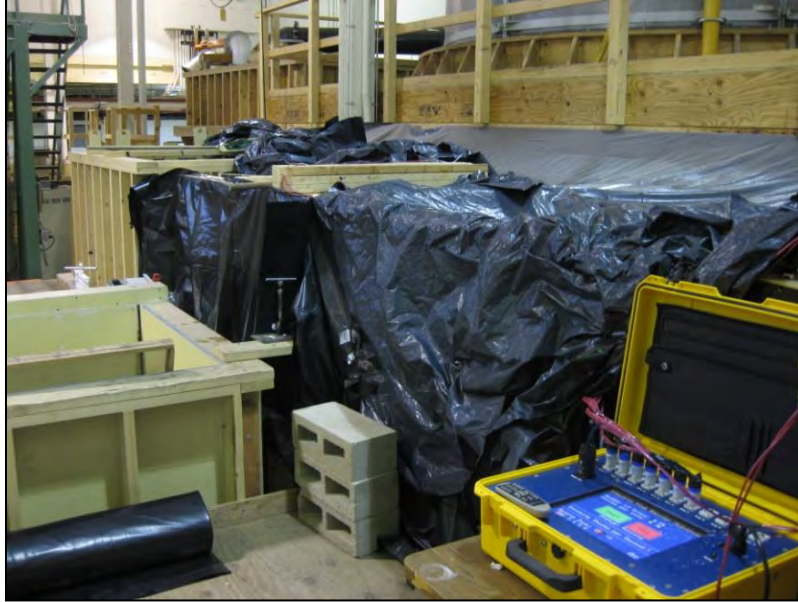
Figure 6.—For some tests, the flume was covered by black plastic to simulate dark conditions.
