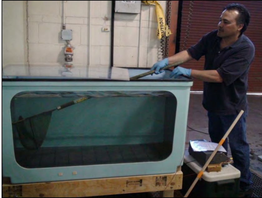
Figure 1.—Laboratory test tank with flat plate metal electrodes covering the full dimension of the side of the tank.
