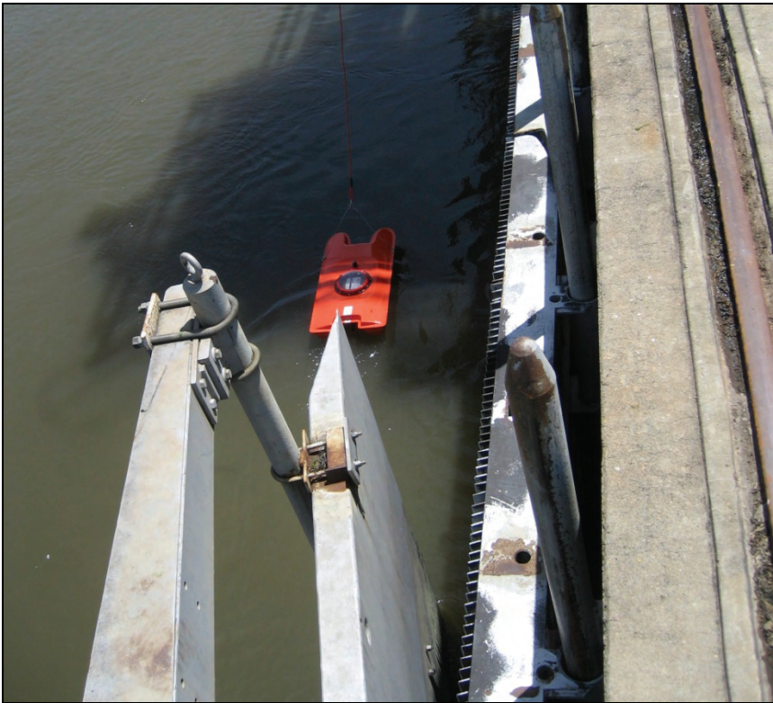
Figure 4.—OTT Qliner current profiler floating upstream of a bypass intake.
