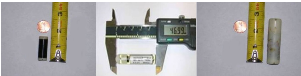
Figure 2.—Acoustic transmitters (Sonotronics, Inc., Tucson, Arizona) used for tracking striped bass at the Tracy Fish Collection Facility (Bureau of Reclamation, Byron, California). From left to right: IBT-96-5, IBT-96-9 (Sonotronics 2010), and CHP-87-S.
