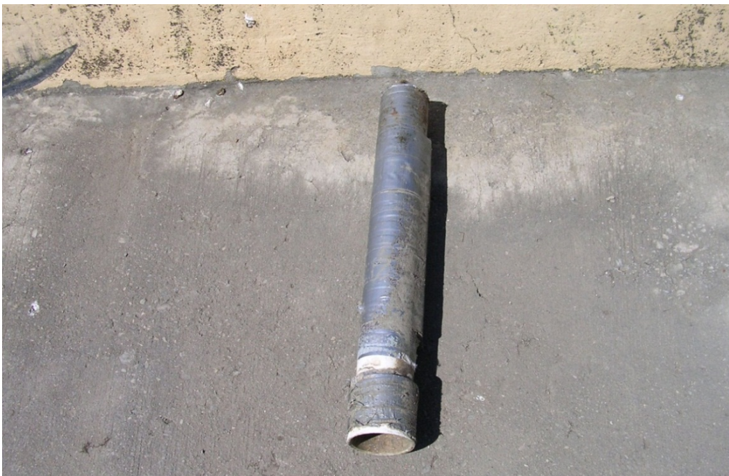
Figure 6.—Example of Model SUR-1 submersible ultrasonic receiver used for automated passive detection of acoustically tagged striped bass at the Tracy Fish Collection Facility (Bureau of Reclamation, Byron, California).
