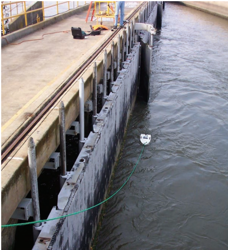
FIGURE 9.—The BoogieDopp was positioned upstream from the intake entrance to document near-field approach velocity conditions.
