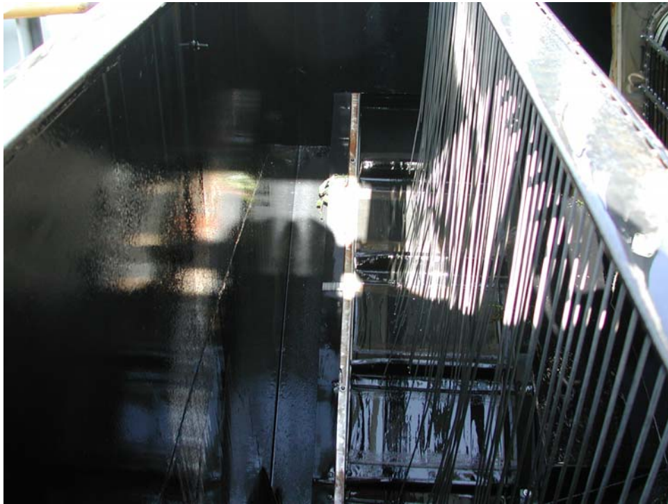
FIGURE 4.—The stainless steel tines were lowered further into the hopper and closer to the conveyor belt to intercept and drop more debris onto the conveyor.
