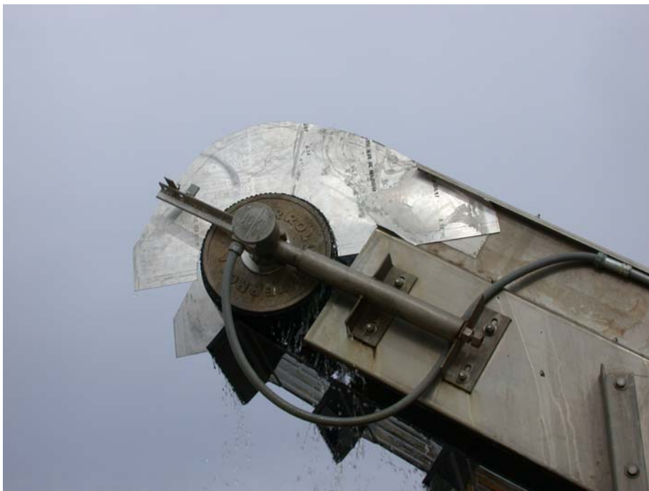
FIGURE 2b.—After: Sheet metal guides keep debris on conveyor to the end of the belt so that it is collected.
