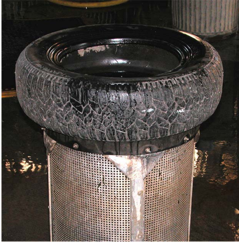
FIGURE 4.—Car tire used to seal the top rim of the 10-minute-count screens.
