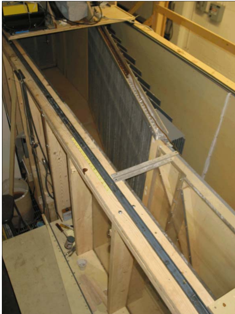
FIGURE 6.—Photograph of 1:6 Froude-scale physical model of a single TFCF primary bypass with an approach louver line.
