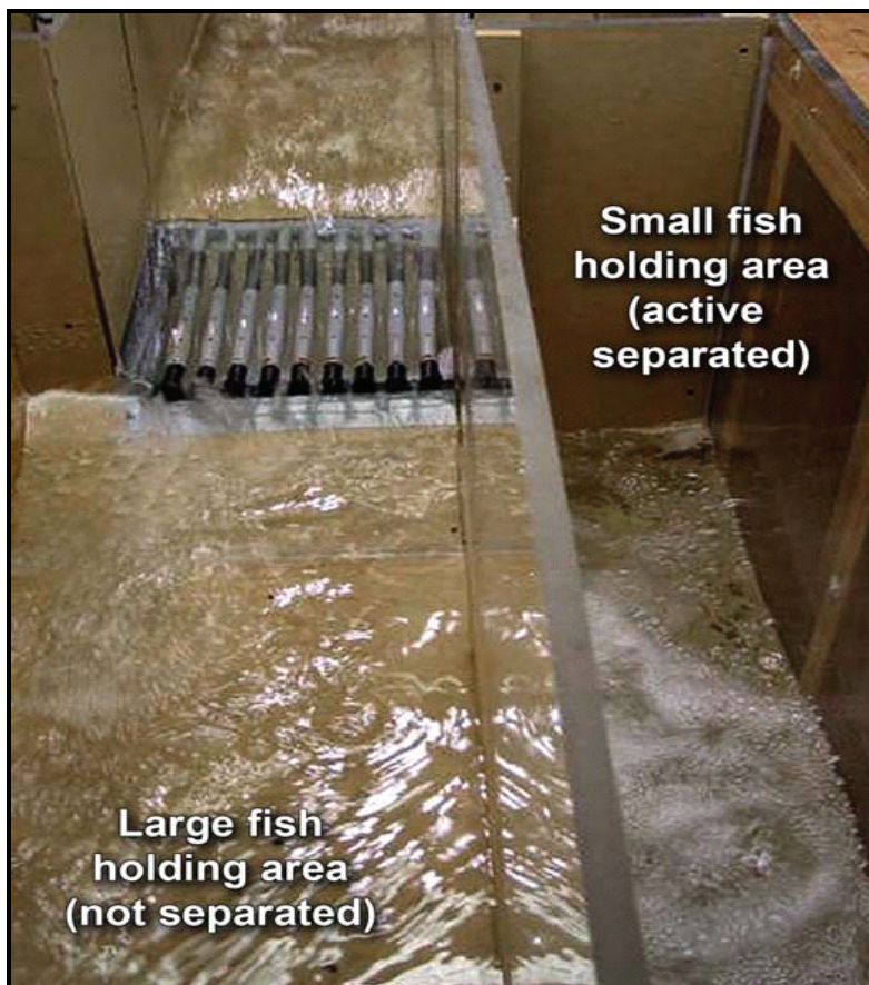
FIGURE 9.—Active separator divider wall showing separate holding areas for actively separated small fish and raceway area for large fish that are not separated.
