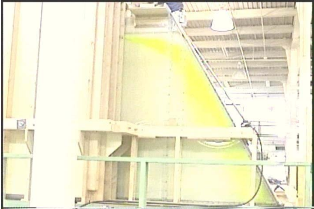
Figure A2-3.—Baseline Flow Visualization. Model operated at a flow depth of 20 feet and a discharge of 40 ft 3 /s.
