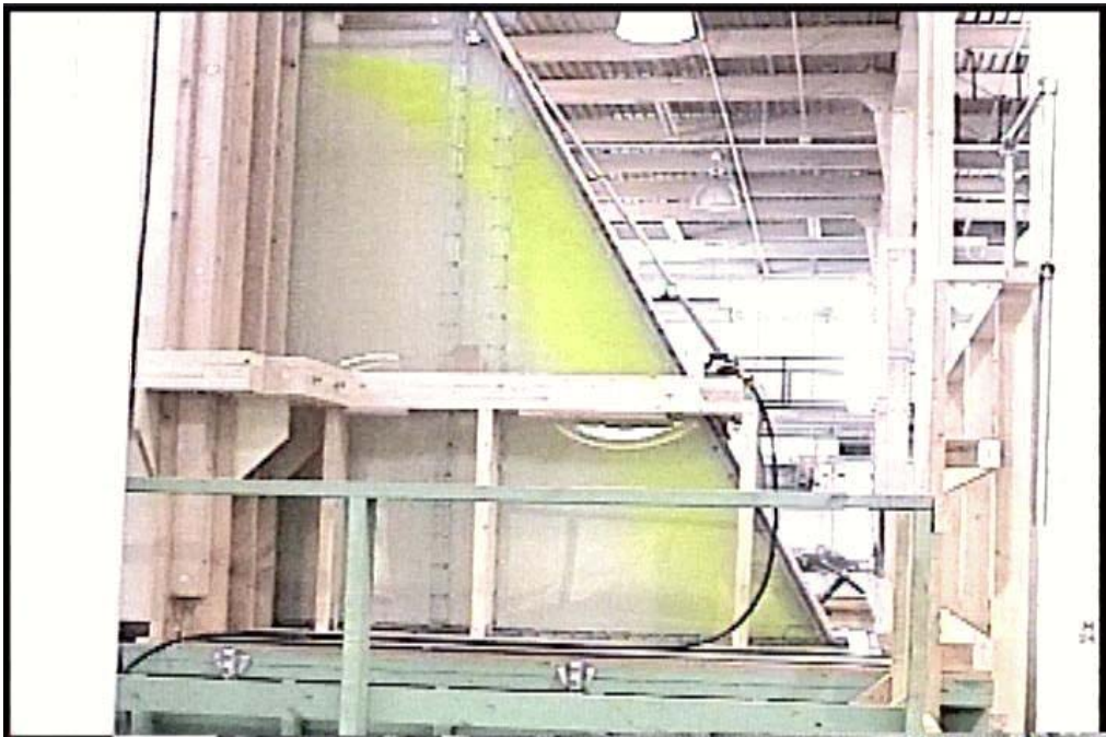
Figure A2-2.—Baseline Flow Visualization. Model operated at a flow depth of 20 feet and a discharge of 20 ft 3 /s.
