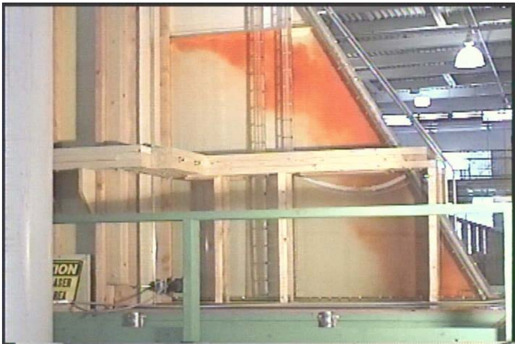
Figure A2-4.— Final Flow Visualization testing for step-widened, vertical choke transition bypass modifications. Model operated at a flow depth of 16 feet and a discharge of 20 ft 3 /s.
