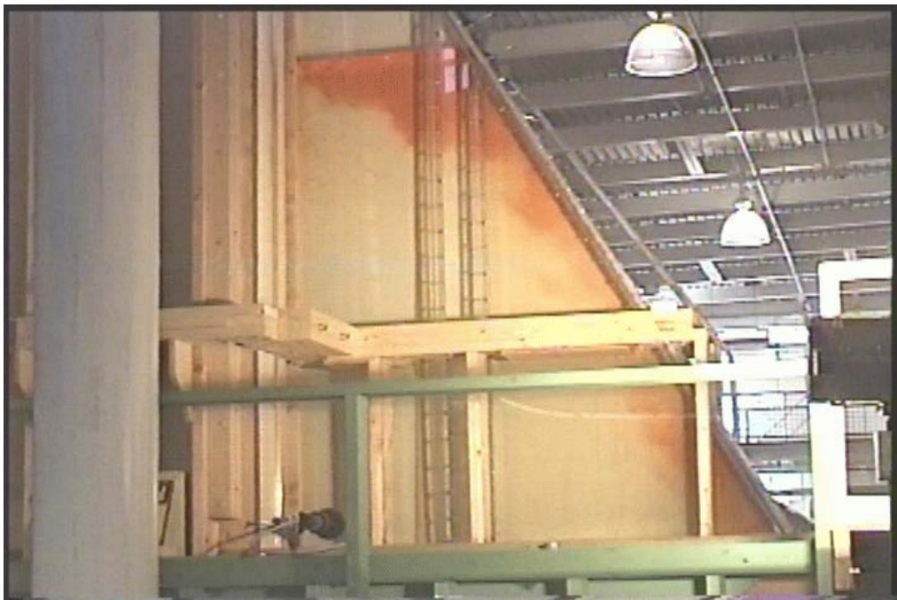
Figure A2-6.—Final Flow Visualization testing for step-widened, vertical choke transition bypass modifications. Model operated at a flow depth of 20 feet and a discharge of 40 ft 3 /s.
