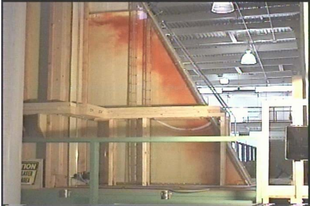
Figure A2-5.—Final Flow Visualization testing for step-widened, vertical choke transition bypass modifications. Model operated at a flow depth of 20 feet and a discharge of 20 ft 3 /s.
