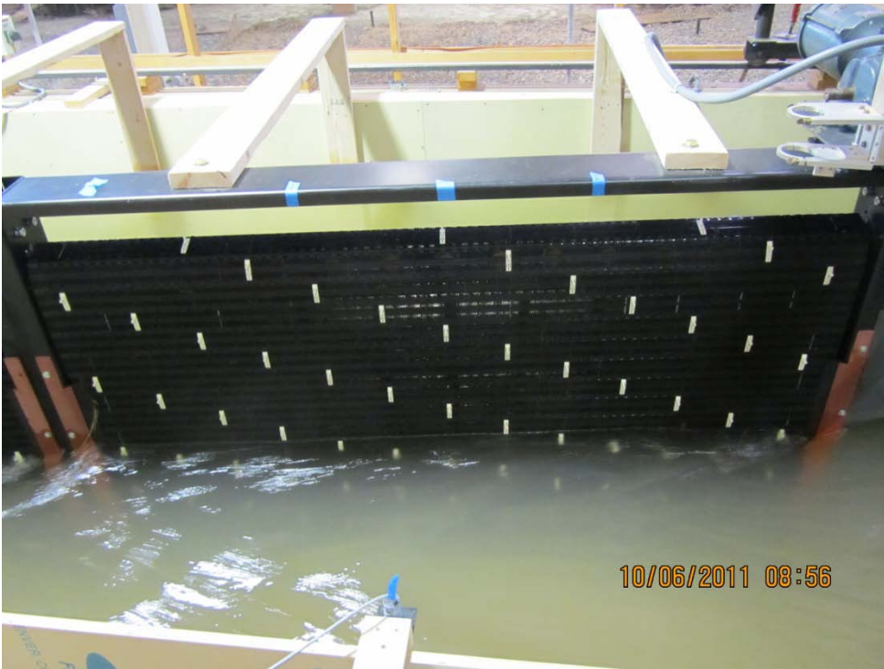
Figure A-16 - Debris peg layout on upstream side of screen (flow from right to left)
