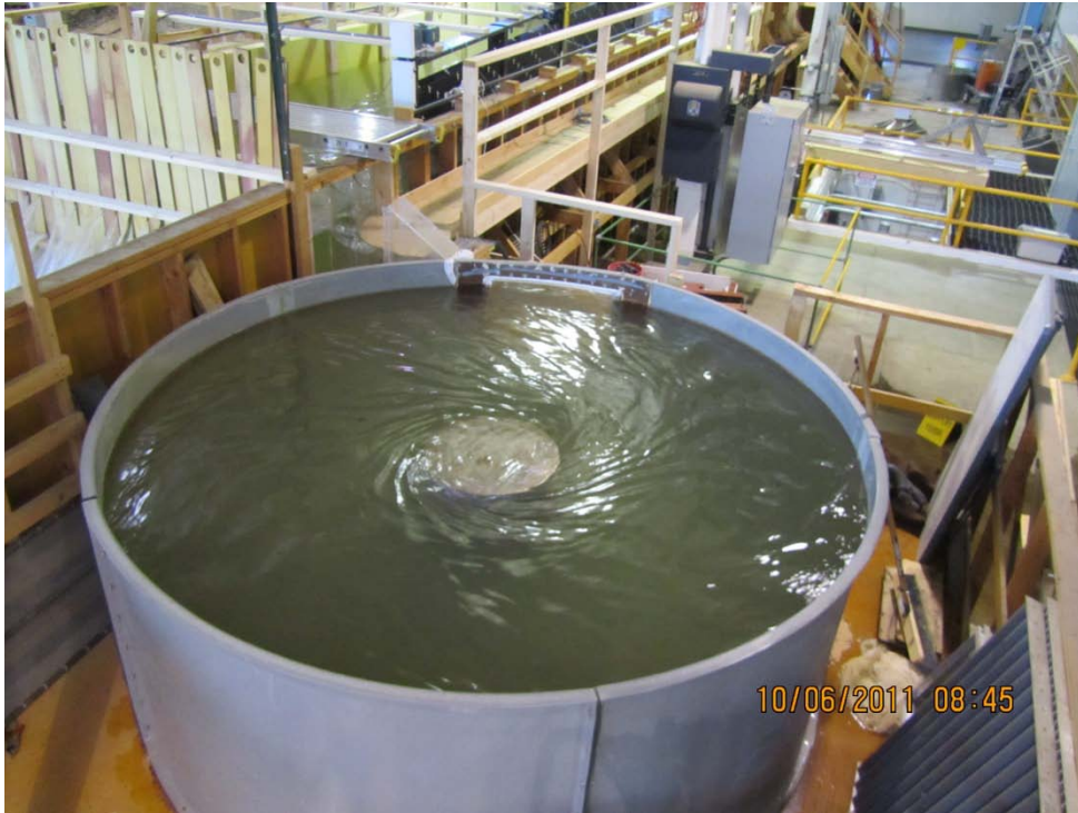
Figure A-3 - Holding tank during a test (flow entering the tank from the top)
