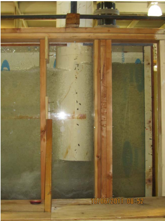
Figure A-12 - Inflow 4 into the clean water bypass (flow from right to left)
