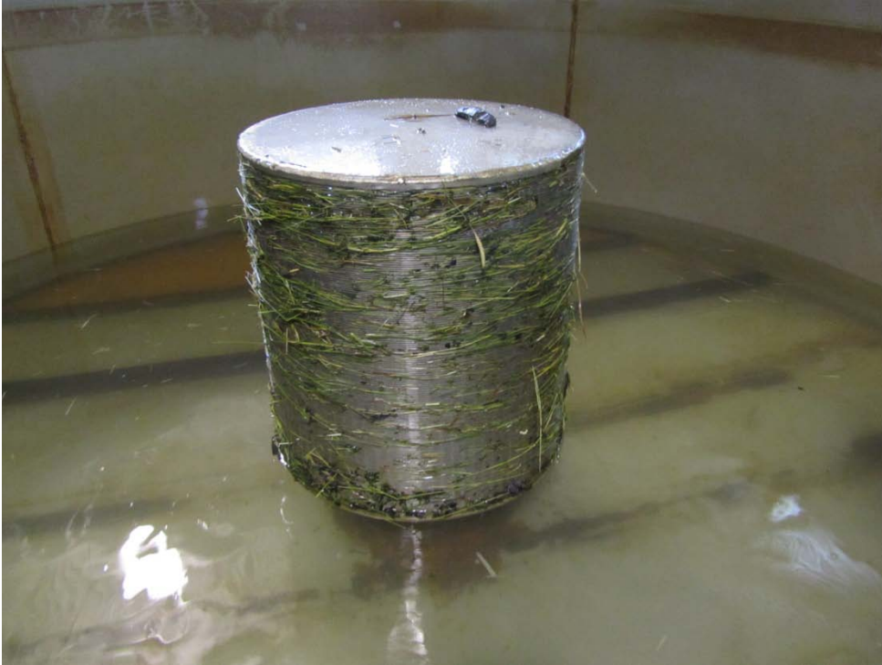
Figure A-11 - Hay and woody debris in the holding tank after a test is complete.
