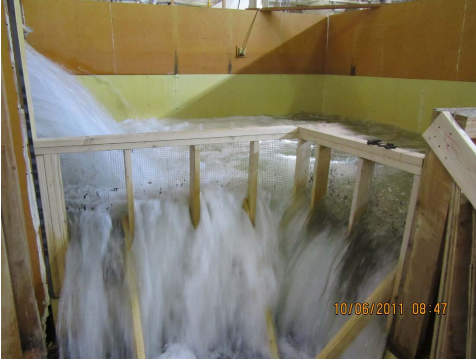
Figure A-5 - Tailbox during a test (flow towards reader)
