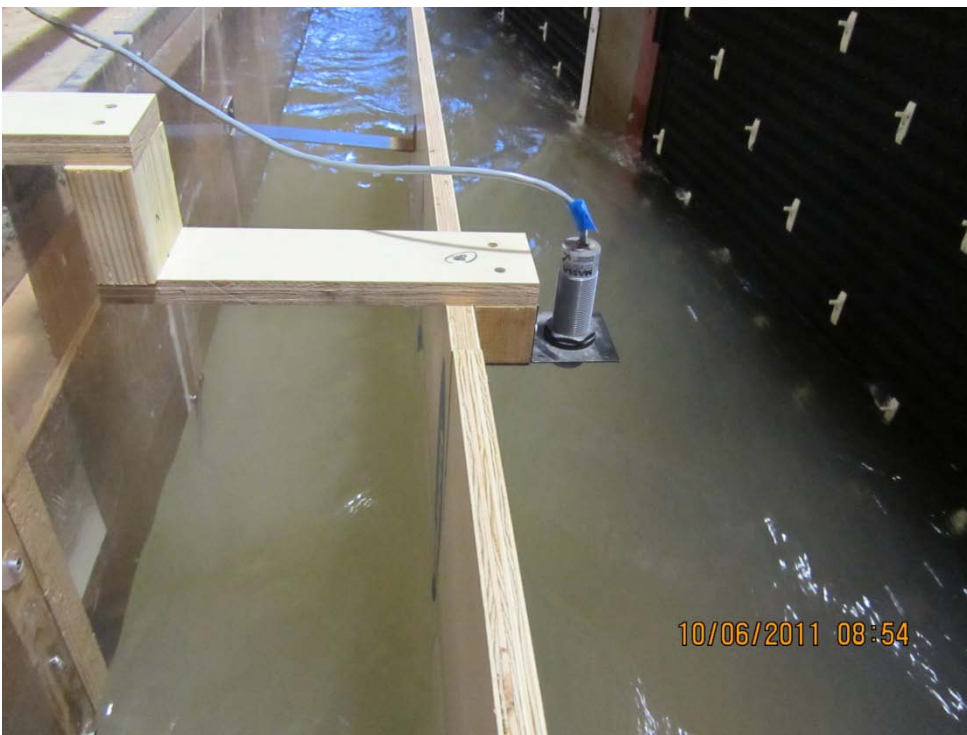
Figure A-14 - Ultrasonic downlooker to determine flow depth (1 of many)
