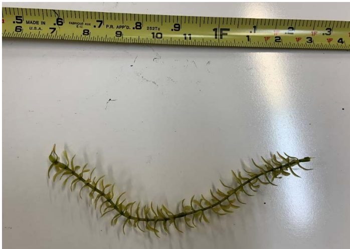
Figure 4. An example of the plastic aquarium plant strings that were used to represent the submerged aquatic vegetation. The aquarium plant strings varied in length from 3 to 10-inches (model scale, equivalent to 12 to 40 in. prototype scale).
