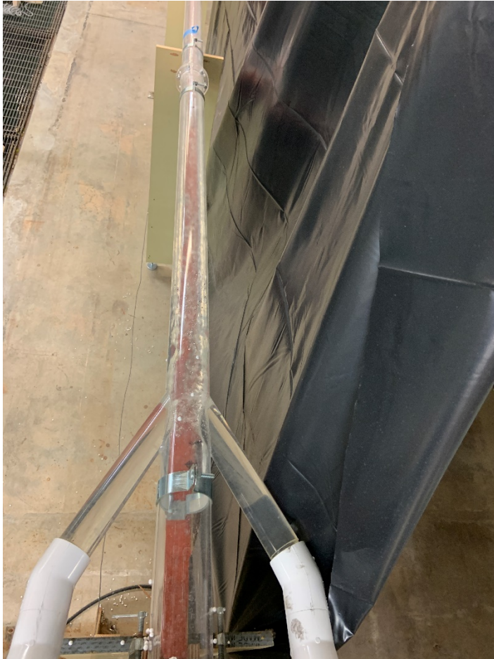
Figure 2. Top down view of the auxiliary flow manifold (direction of fish release is from the bottom of the photo to the top).
