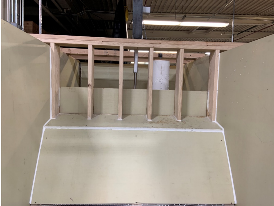
Figure 6. The downstream slide gate looking upstream. This allows for control of the tail water elevation to match simulated river water surface elevations over the desired range of operation.
