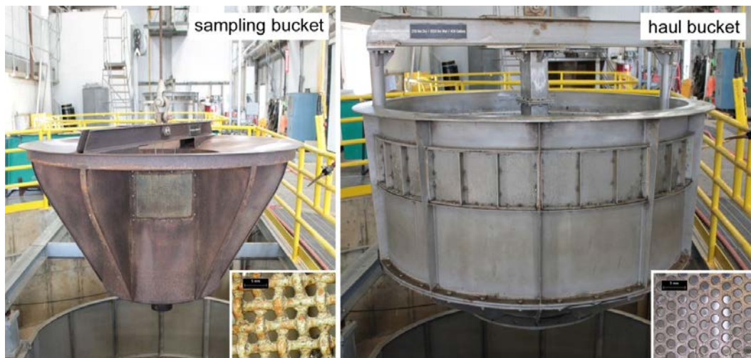
Figure 9 Fish bucket: the sampling bucket (left) and the haul bucket (right) used at the Tracy Fish Collection Facility
