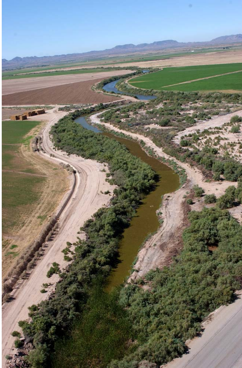
Figure 7. Invasive Salvinia growing in canal affecting water conveyance. Photography courtesy Denise Hosler, Reclamation.
