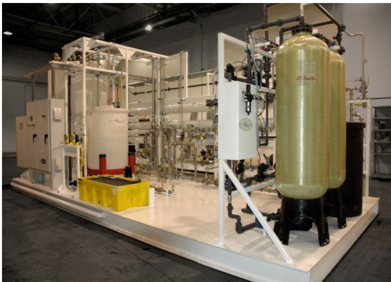
FIGURE 2.24 NEW JERSEY ARROW PROJECT FOR REJECT RECOVERY
