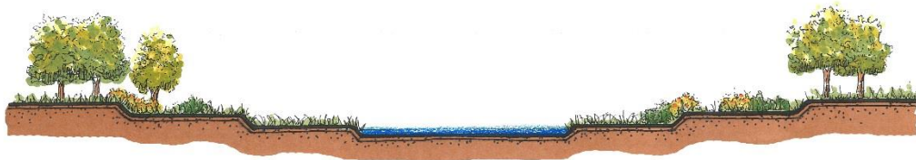
Figure 24. Floodplain Reclamation Typical Section
