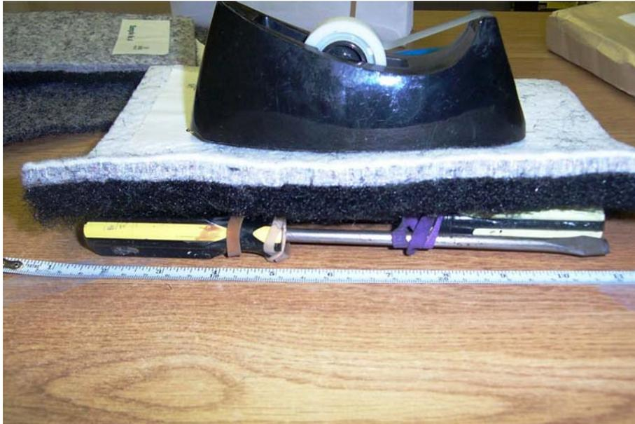
Photo 3: Three Layer Geosynthetic Filter
