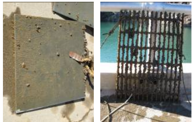
Figure 2. Flame sprayed zinc metallizing contrast between plates (minimal flowing conditions) and grates (flowing conditions).
