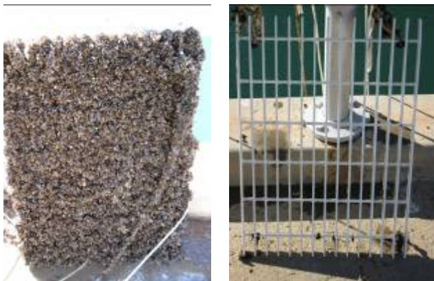
Figure 1. – Uncoated steel grate after 7 months (left). Non-toxic foul release coated steel grate (right).
