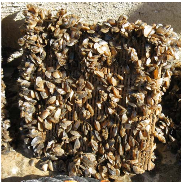
Figure 2. - Quagga mussel settlement on Cu-Ni (90-10) wedge wire screen sample.
