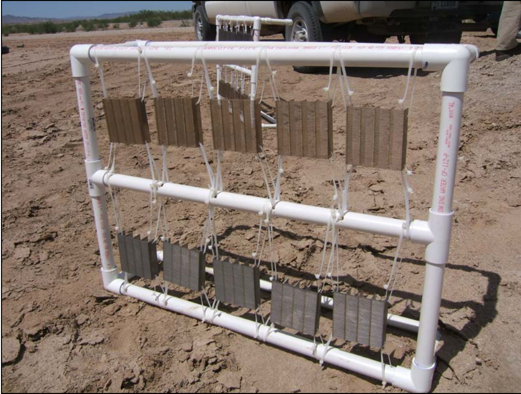
Figure 7. Screen coupons attached to PVC frame using nylon zip-ties prior to deployment.
