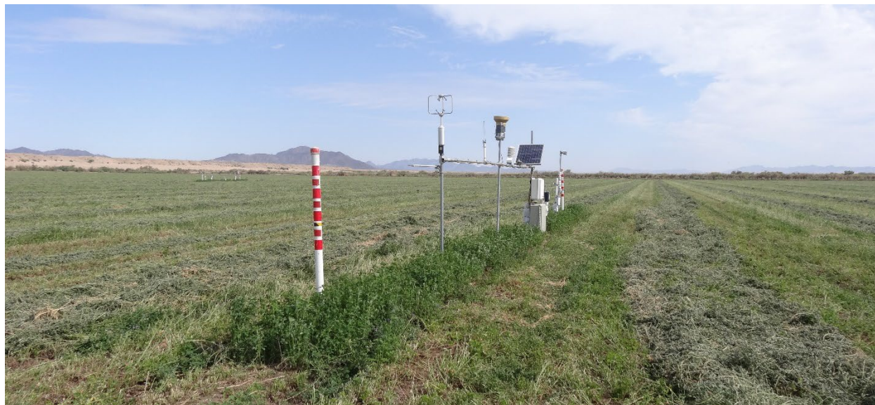
Figure 24 Photo of Eddy Covariance, Surface Renewal Systems and Other Monitoring Equipment (credit, B. Barker).
