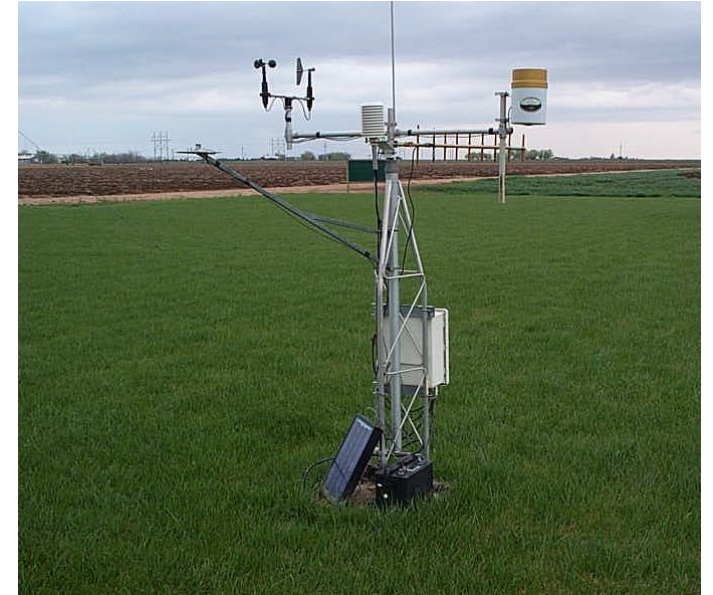
Automated agricultural weather station, Bushland, TX. Photo courtesy of Tom Ley.
