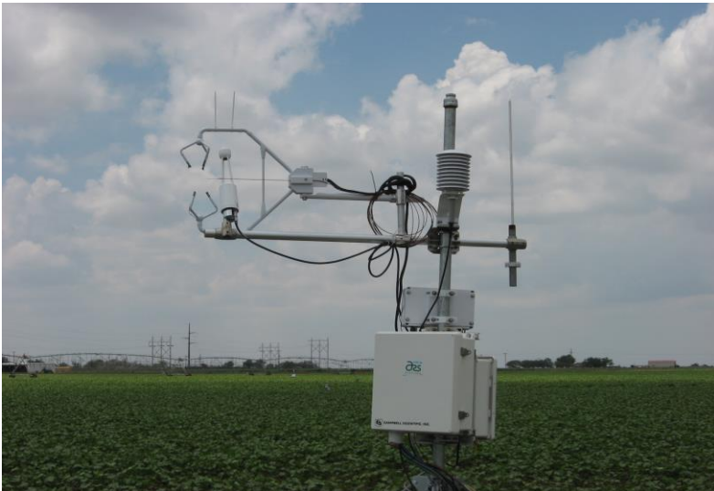
Eddy Covariance Station, USDA ARS Conservation and Production Research Laboratory, Bushland TX. Photo courtesy of Tom Ley.
