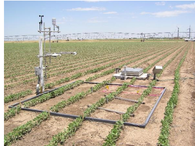
3m x 3m weighing lysimeter with monolithic core at USDA ARS Conservation and Production Research Laboratory, Bushland TX. Photo courtesy of Tom Ley.
