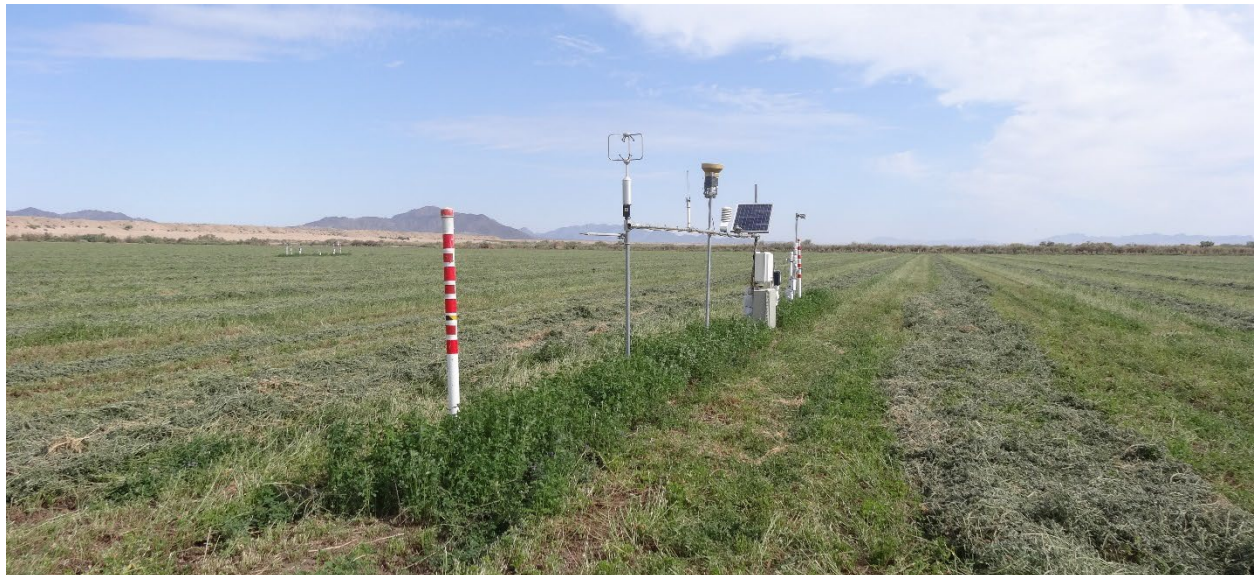
Figure 24 Photo of Eddy Covariance, Surface Renewal Systems and Other Monitoring Equipment (credit, B. Barker).
