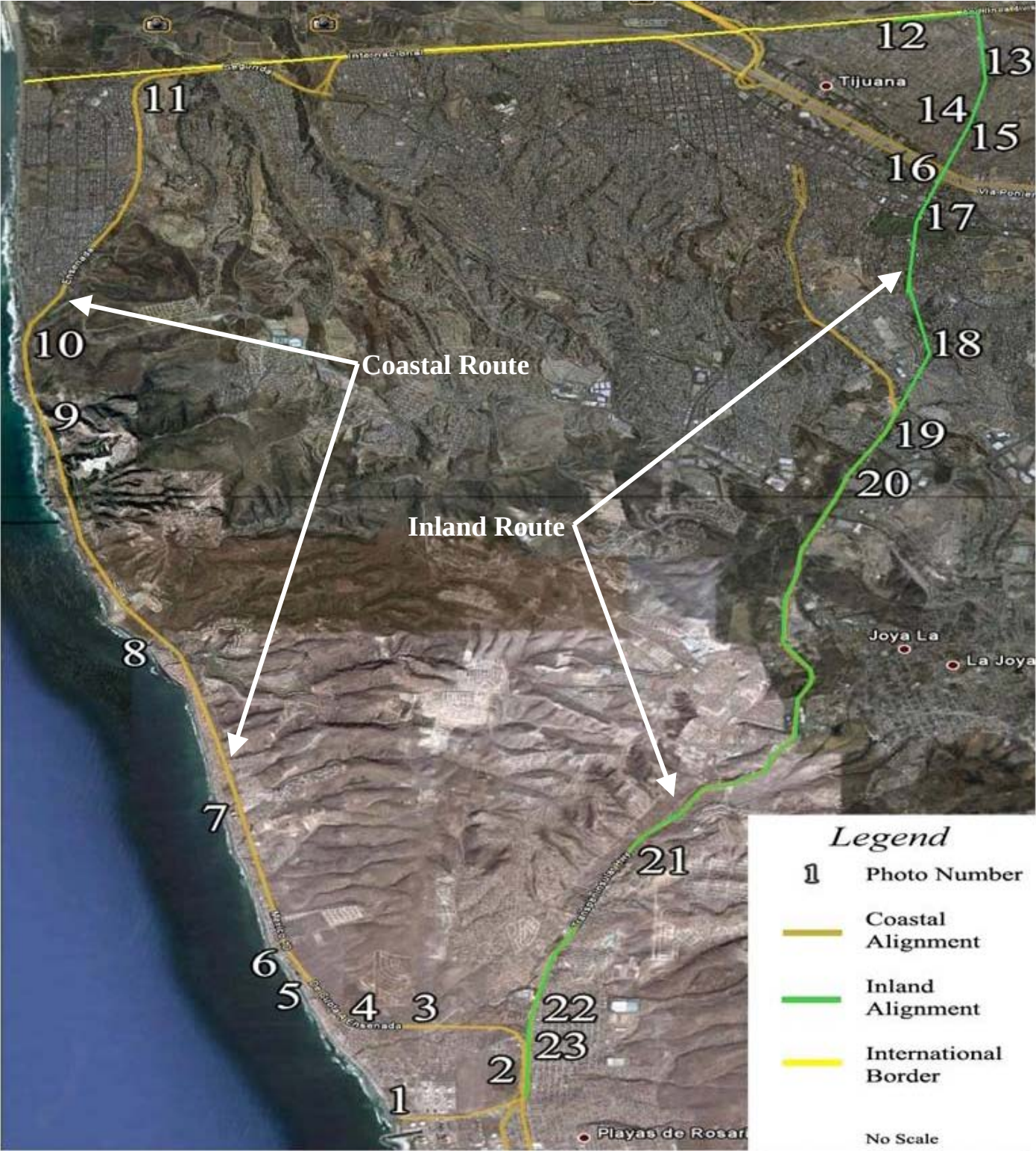
Figure 2-7: Treated Water Pipeline Alignment Alternatives
