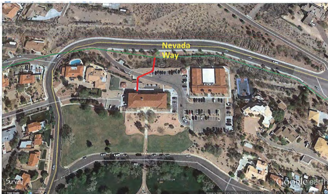
Figure 3. Fiber optic cable leg to be replaced (depicted in red), connecting to 1200 Park Street building.
