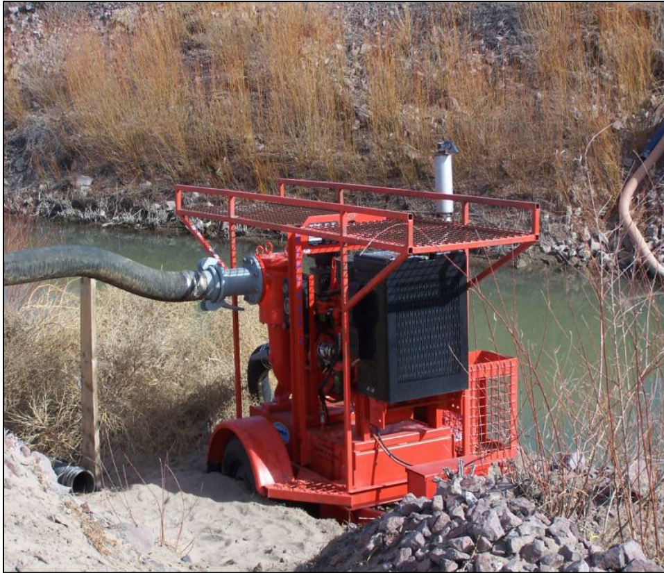
Figure B-3. Water for vehicle cleaning was pumped from conveyance channel at Socorro, New Mexico field site (Reclamation).
