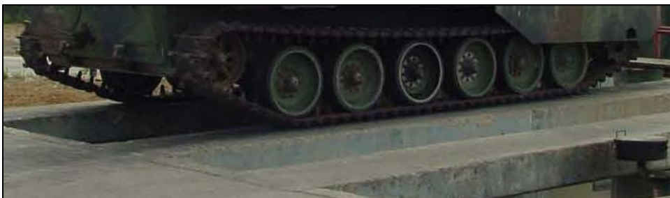
Figure A-12. All tracked land vehicles share many common components such as tracks, rollers, idlers, tensioners, and sprockets (U.S. Department of Defense).
