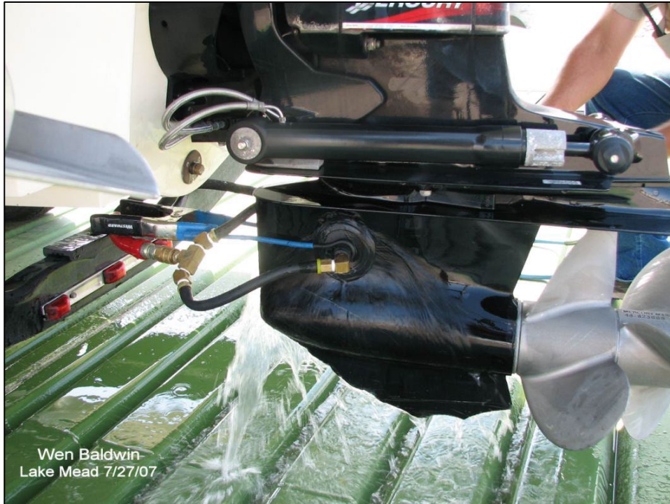
Figure B-5. Inboard/outboard engine flushing (Pacific States Marine Fisheries Commission/Wen Baldwin).
