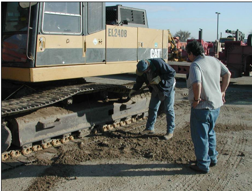
Figure 4. Pre-cleaning heavy accumulations of soil from tracked equipment (Reclamation/Fred Nibling).
