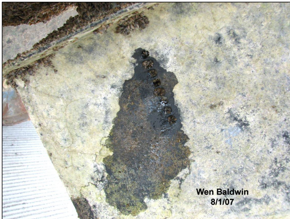
Figure A-2. Closeup view of outboard motor shaft housing with adult quagga mussels living inside the engine (Pacific States marine Fisheries Commission/Wen Baldwin).
