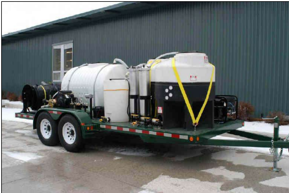
Figure B-4. Trailer-mounted washing system field tested by Forest Service for cleaning land use vehicles and other equipment (U.S. Department of Agriculture, Forest Service photo).
