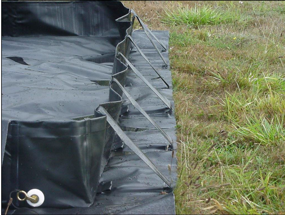
Figure B-2. High-wall portable berm with wall supports in place. High-wall berms might offer better overflow protection when conducting equipment washing. Remove the wall supports on one side to move equipment onto the berm. All wall supports can be removed, and the entire berm rolled up for easy moving and storage. Bung openings can be positioned to fit specific need when ordering from the company (Reclamation/Joe DiVittorio).
