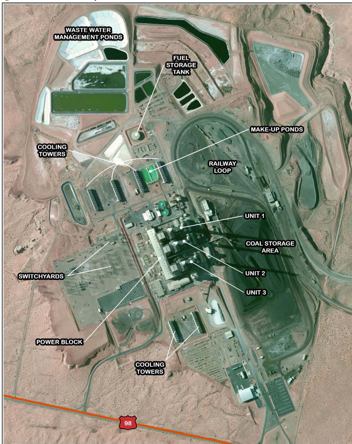
Figure 4 - NGS Plant Layout.
