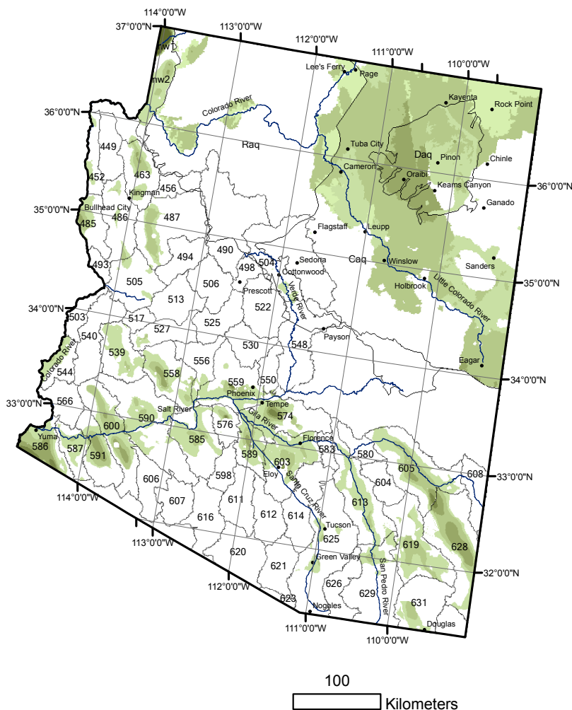
Figure 26: Estimated well development capital costs for desalination at 10,000 m 3 /d and 50,000 m 3 /d where brackish groundwater was predicted to exist within 20 km of annual average wind class 3 or greater in Arizona.
