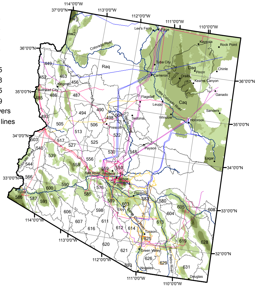
Figure 20: Estimated capital costs for desalination at two desalination plant capacities using grid electricity where brackish groundwater resources were predicted to exist in Arizona.
