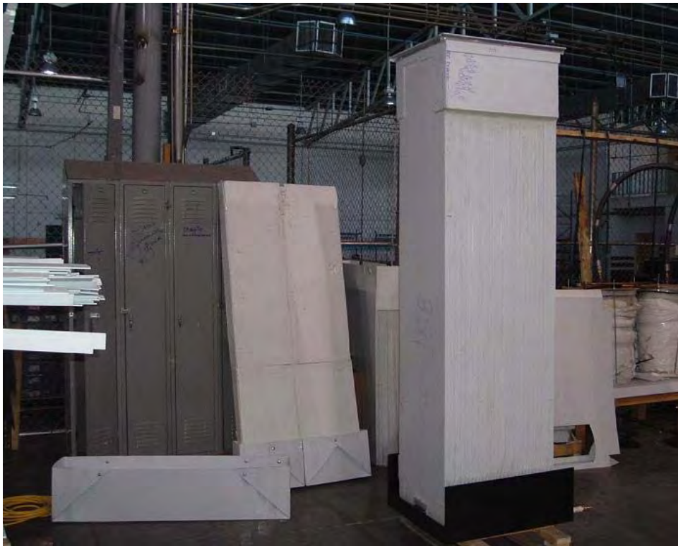
Figure 4. Tower sections fitted with gauze.
