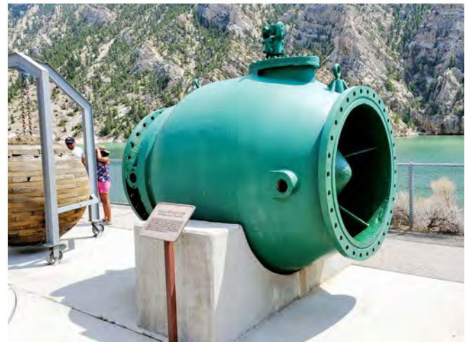
Balanced Plunger Hydraulic Valve and Ball Plug | Image: Ayres
