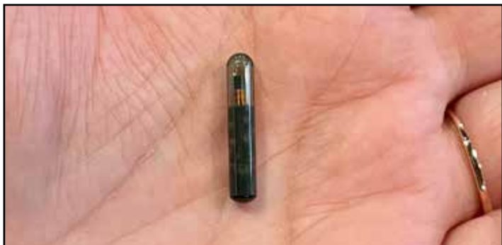
A Passive Integrated Transponder tag used to track bull trout in the St. Mary River and its tributaries in northwestern Montana.
