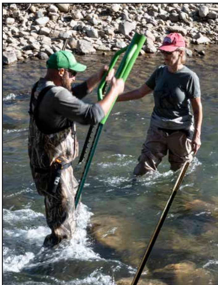
Jacob Bradshaw, Reclamation natural resources specialist and Lauri Teig, Reclamation environmental specialist, pound T-bars into the riverbed to secure a cable with an antenna across the river to transmit data of tagged bull trout to a reader system on the bank. USFWS downloads the data from each station to determine information about the health of bull trout populations in the St. Mary River and its tributaries.
