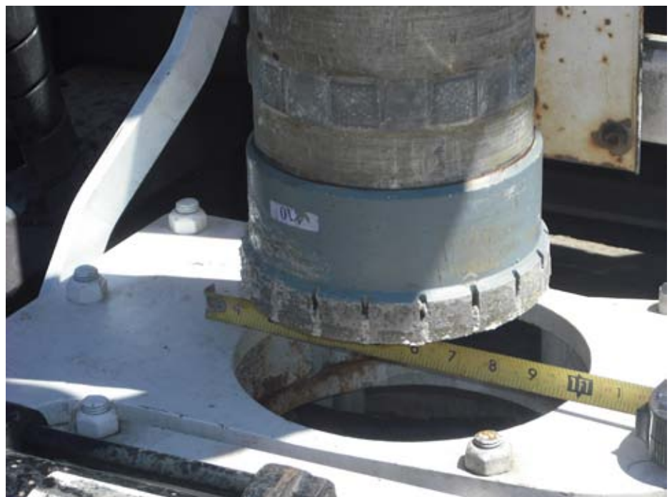
Close up view of the cutting bit (drill bit).
