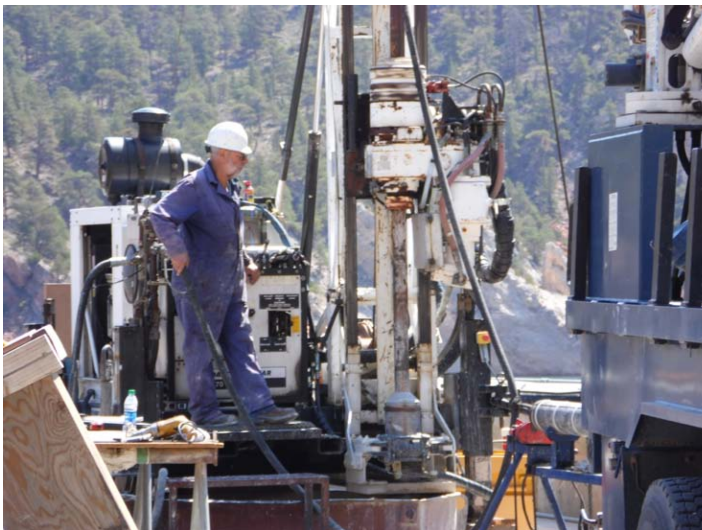
The double-tube core barrel assembly is removed from the bore hole after completing the 5-foot sampled interval and lowered onto the “horses”.
