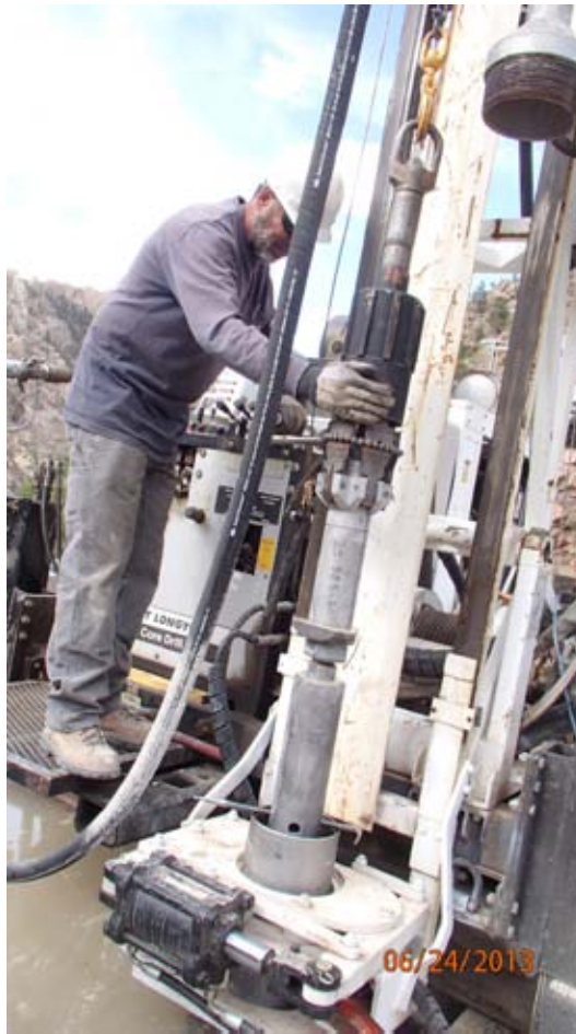
Drill Rig Operator lowers the double-tube core barrel assembly with cutting bit into the hole and prepares to take another 5-foot sample.
