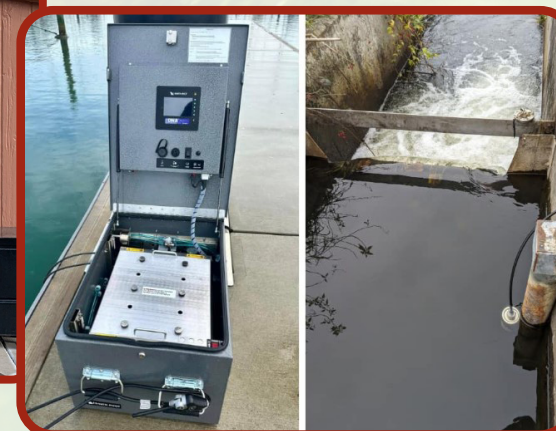
An example of a Smith-Root eDNA autosampler installed in the field (from www.smith-root.com ).
