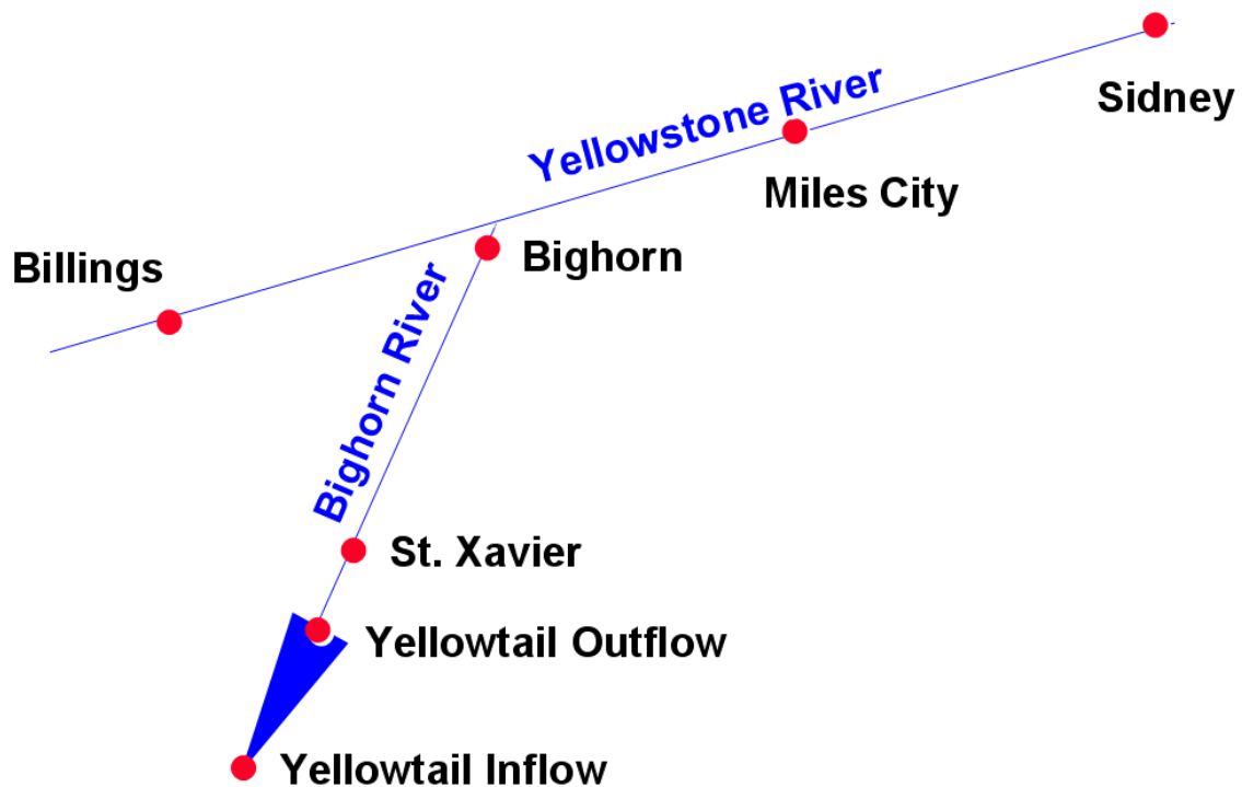
Figure 4. Schematic showing Yellowtail Dam and other computation points within the HEC-ResSim model. Inflows were placed into the model at the Yellowtail Inflow and Billings computation points. Dam outflow was computed at the Yellowtail Outflow computation point and downstream flows were computed at all other locations. Figure is not to scale.
