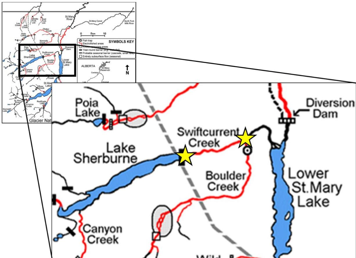
**Figure 9.** Stretch of Swiftcurrent Creek that annually goes dry due to lack of in-stream flow below Lake Sherburne Dam. Yellow stars denote upstream and downstream boundaries of section that is completely de-watered.
