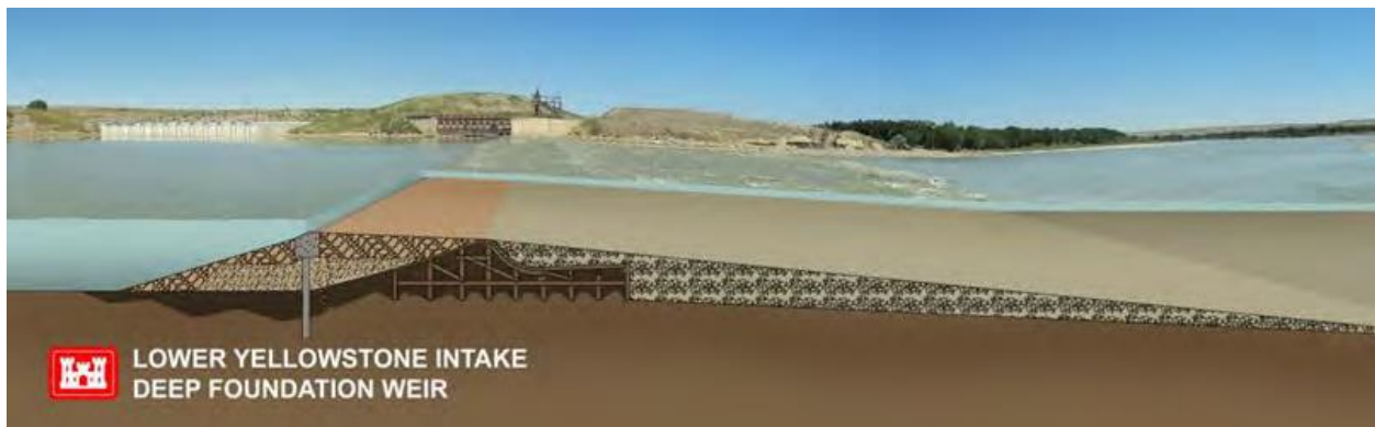
Figure 4. Conceptual model of the replacement weir design in relation to the existing weir (Reclamation and Corps 2016a).
