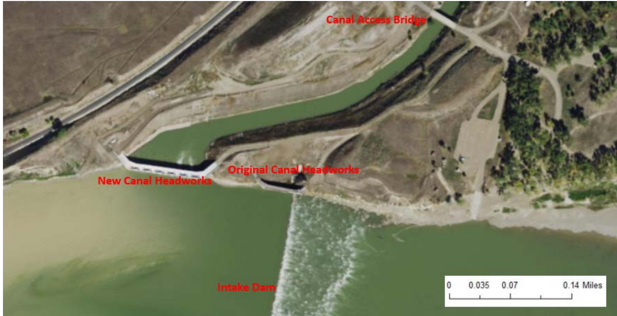
Figure 1. New Intake Canal headworks, original canal headworks, access bridge and low-head diversion dam across the Yellowstone River.
