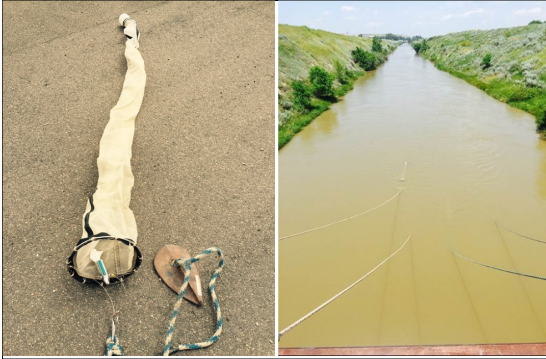
Figure 6a. (Left). Photo of larval fish sampling gear showing plankton trawl net, depressor weight, flow meter, and PVC collecting bucket at the back end of the net.
