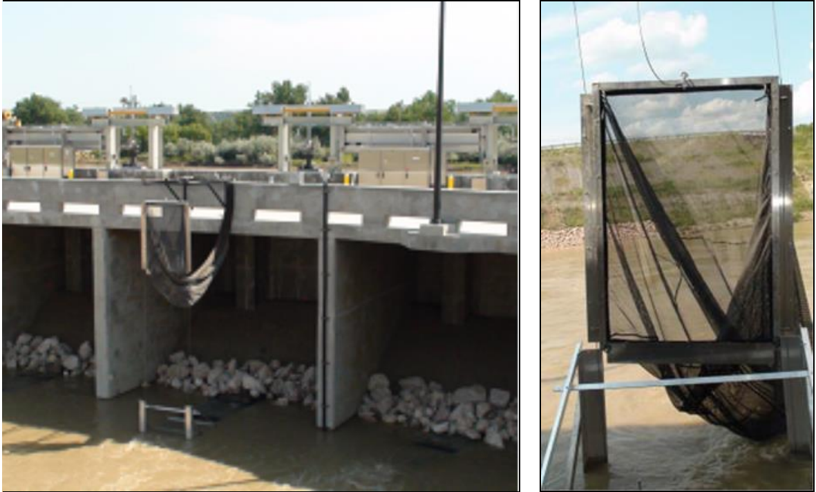
Figure 8. (A) (left) Photo of steel frame structure used to extend the entrainment net frame out about 2.5 meters to line up over the outlet area of the box culvert. (B) (right). Photo of receiving frame structure made from stock plate aluminum constructed onto the outlet of the box culvert to further guide the net into position and hold it in place.
