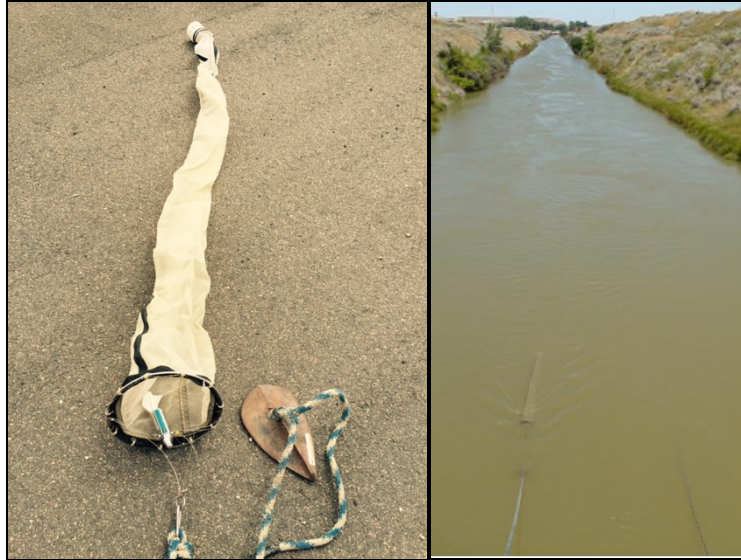
Figure 9 (A) (left). Photo of larval sampling gear showing plankton net, depressor weight, flow meter, and PVC collecting bucket at the cod end. (B) (right). Photo of Intake Canal looking downstream showing the surface sampling net (left) and the rope leading to the bottom sampling net (right).
